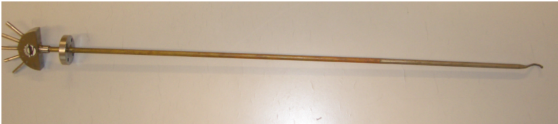
Figure 3: Five-hole SVUSS/5 conical probe
