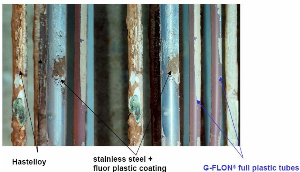
Σχ. 4.3: Σύγκριση διαφόρων υλικών σωλήνων Πηγή: Experiences with Heat Recovery Systems for Lignite Power Plants to increase the efficiency and to reduce CO 2 Emissions , Adamczyk, 2001
