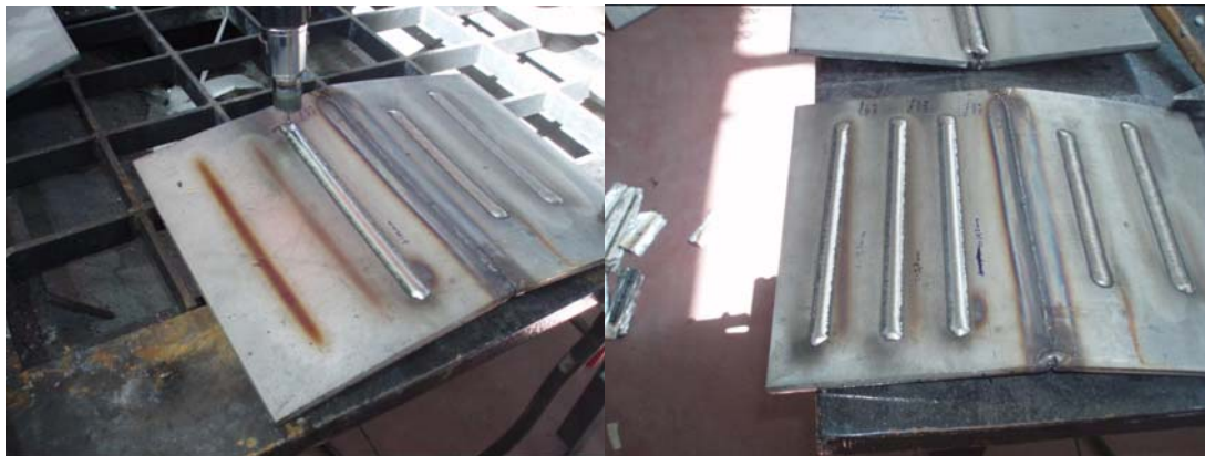
Figure 4.4 Bead-on-plate tests on scrap plates of AISI 316L
