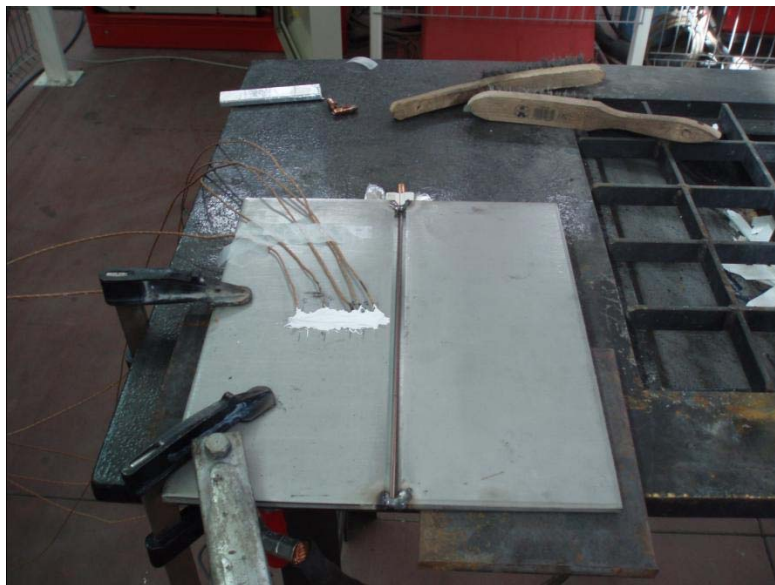
Figure 4.6 Temperature measurements in A-series plates with the use of Type-K thermocouples
