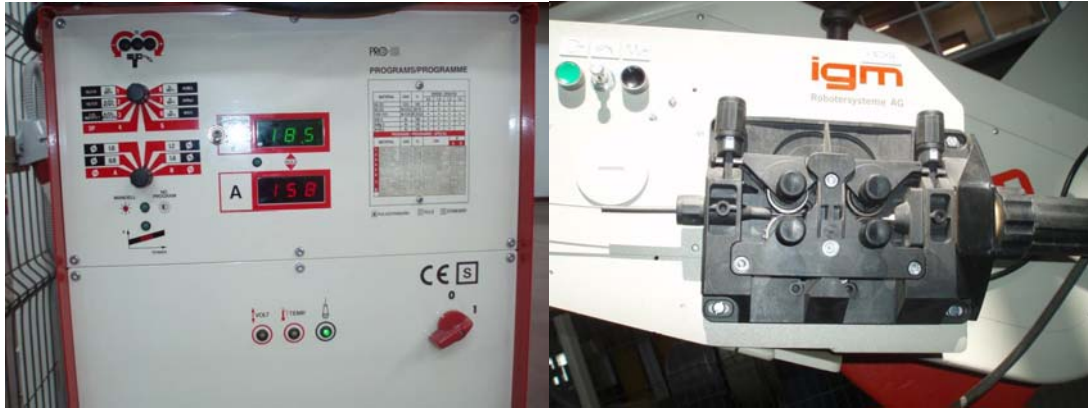
Figure 4.2 a) The constant voltage GMAW machine and b) the wire-feeder attached to the robotic arm
