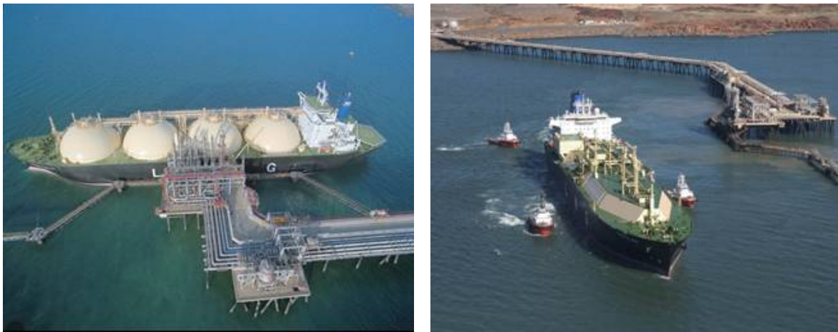
Fig. E.6 LNG carrier with Moss Spherical tank containment system and LNG carrier with Membrane tank Containment system [35].
