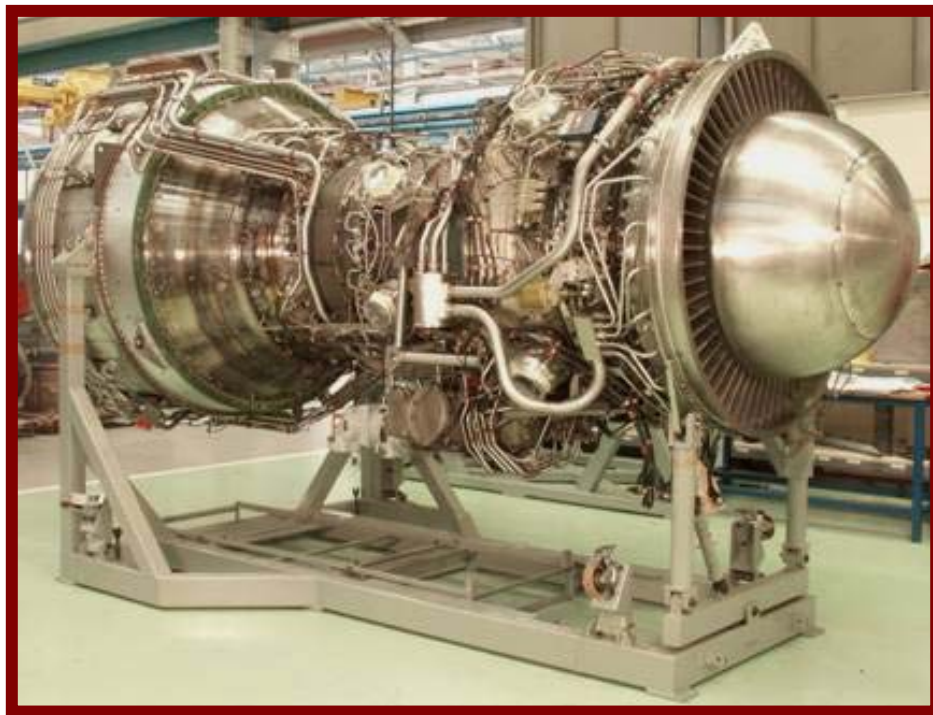
Fig. 2.2.3 Rolls Royce MT30: 36 MW flat rated at 26°C, 42% thermal efficiency, 201 g/kWh on gas, Dual fuel capable [41].
