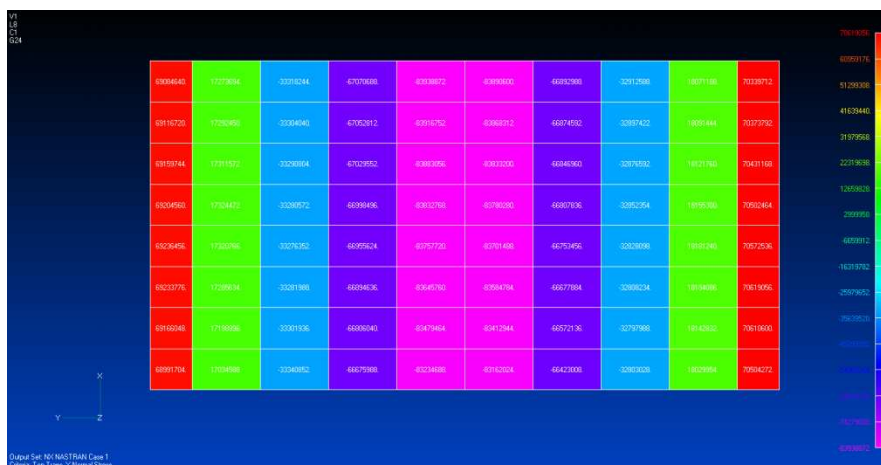
Fig.8.1.2.2 - \sigma_y stress in Bottom plate for Scenario A
