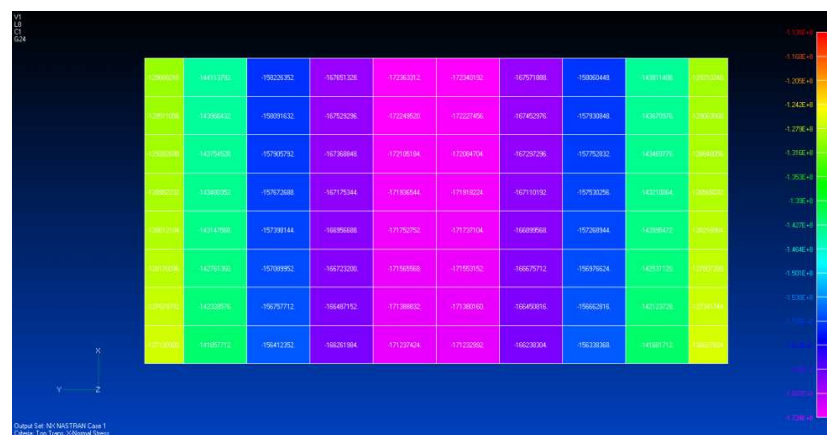
Fig.8.1.2.1 - \sigma_x stress in Bottom plate for Scenario A
