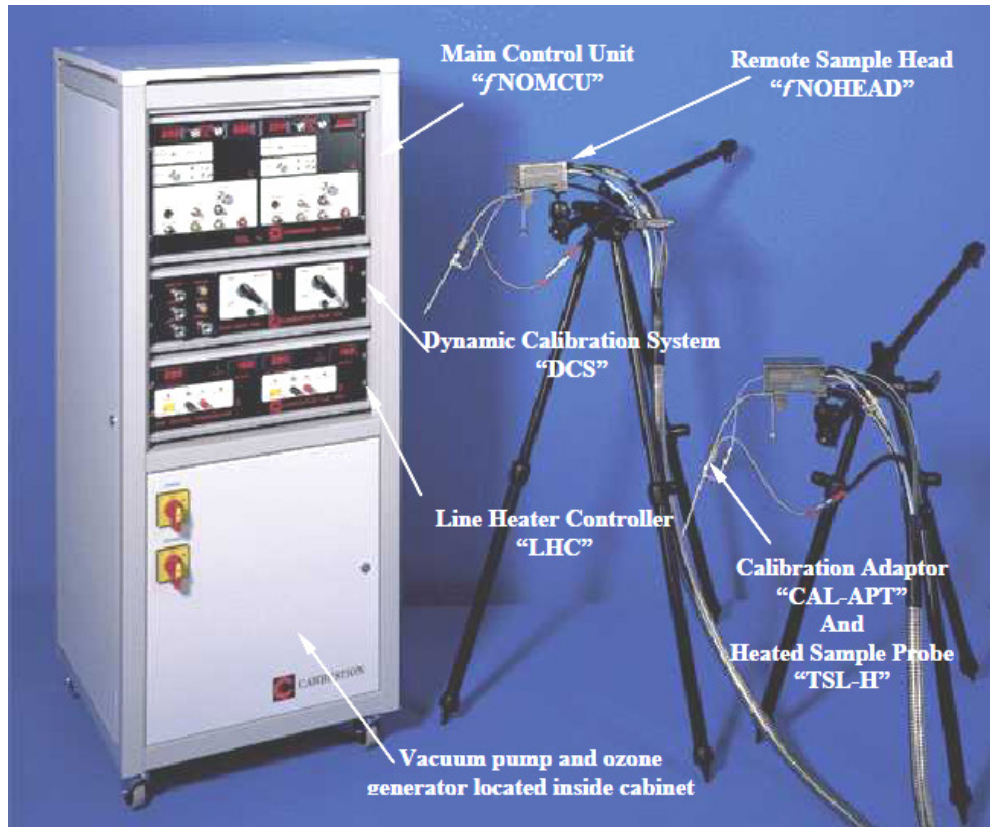
Figure 1: The main items of a f NOx400 Fast CLD system.
