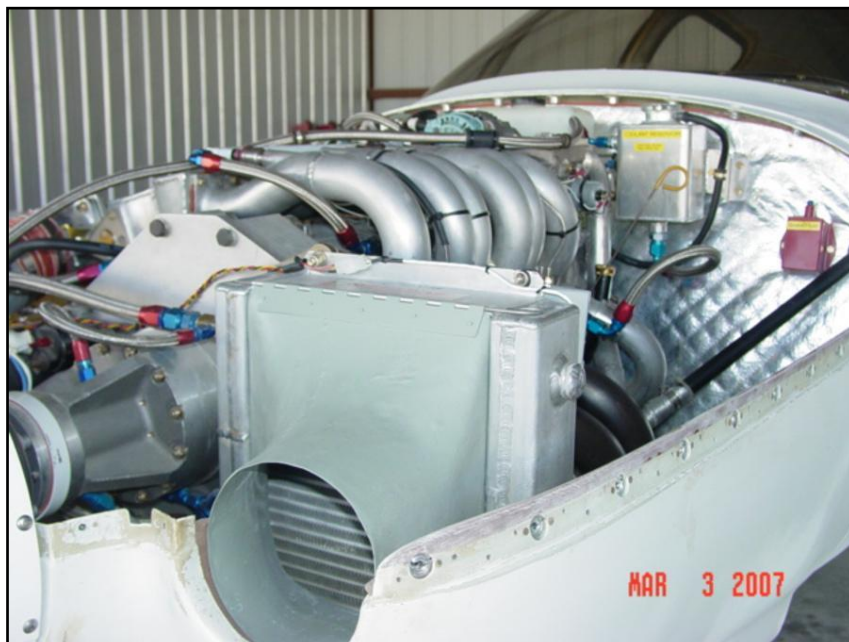
Mark Steitle Lancair ES Mazda three rotor left side.
