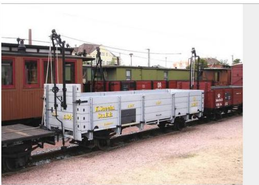
A Class Ow goods wagon on the Saxon narrow gauge railways with Heberlein brakes
