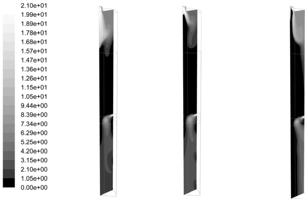
Fig. B4.5: Simulation results of the VVA facility for wall boundary conditions of constant temperature, Oxygen contours (% vol. dry) for (a) case A0, (b) case A1, (c) case A2
