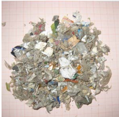
Fig. 4.11a: Typical SRF sample from MSW Fig. 4.11b: SRF fractions after manual sorting
