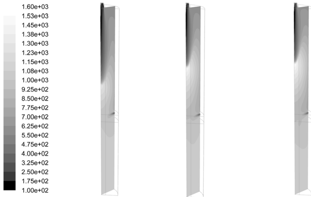
Fig. B4.1: Simulation results of the VVA facility for wall boundary conditions of constant temperature, Temperature contours ( ^{\circ}\text{C} ) for (a) case A0, (b) case A1, (c) case A2
