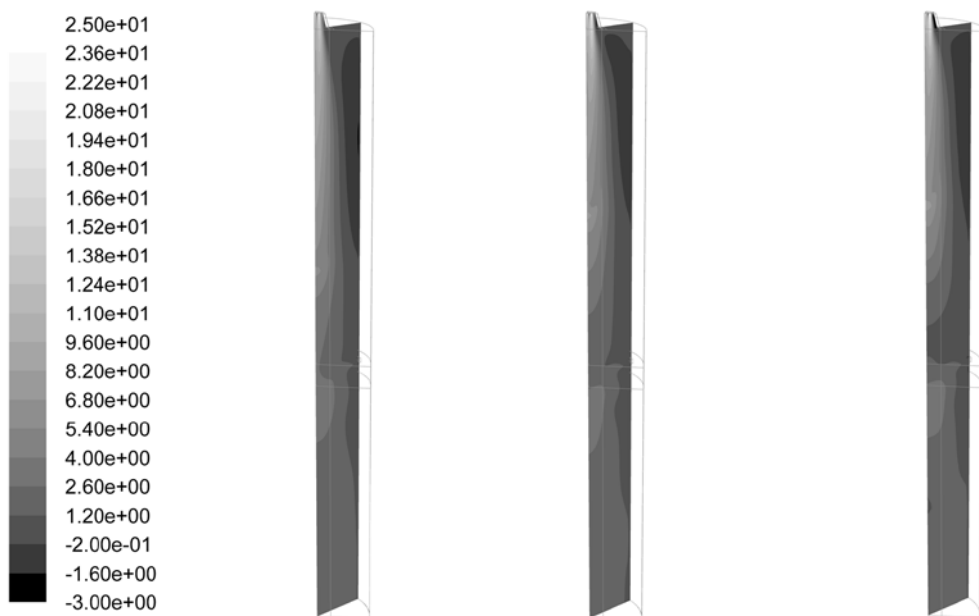
Fig. B4.3: Simulation results of the VVA facility for wall boundary conditions of constant temperature, axial velocity contours (m/s) for (a) case A0, (b) case A1, (c) case A2
