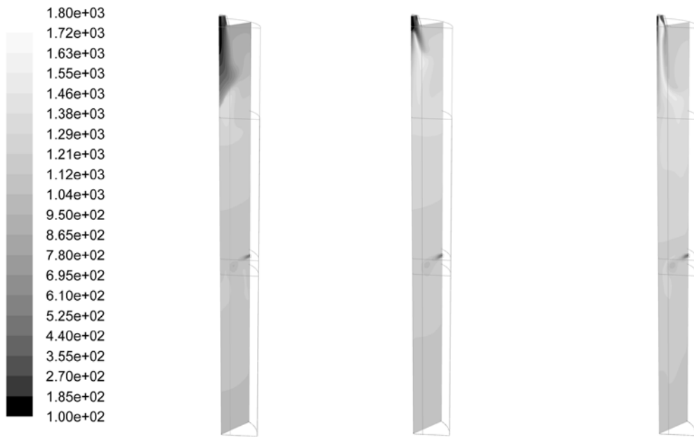
Fig. B4.4: Simulation results of the VVA facility for wall boundary conditions of constant heat flux, temperature contours ( ^{\circ}\text{C} ) for (a) case A0, (b) case A1, (c) case A2
