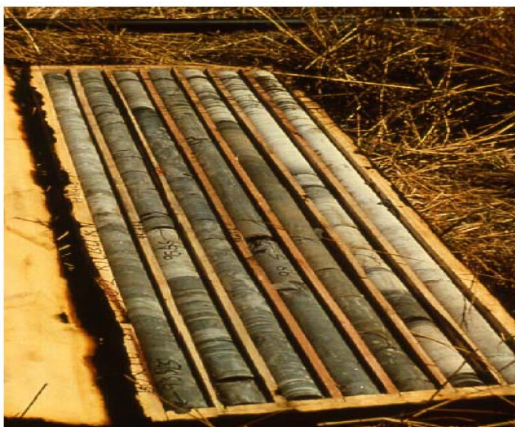
Fig. 6. Freshly drilled sandstones and siltstones from the Drakensberg Pumped Storage Project in South Africa (1972).
