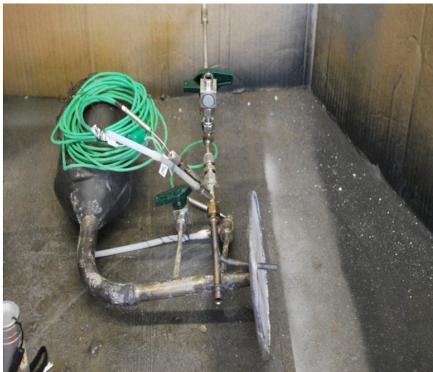
Fig. 4.33: The cutted back side of the second version reformer during reconstruction. It is shown the first dilution system, the postcombustor, the Tmix thermocouple and the position of pressure sensor.
