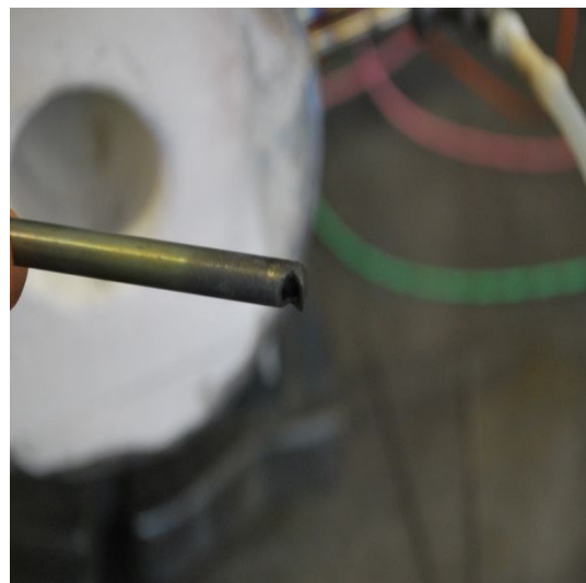
Fig.4.20: The inlet configuration of the probe
