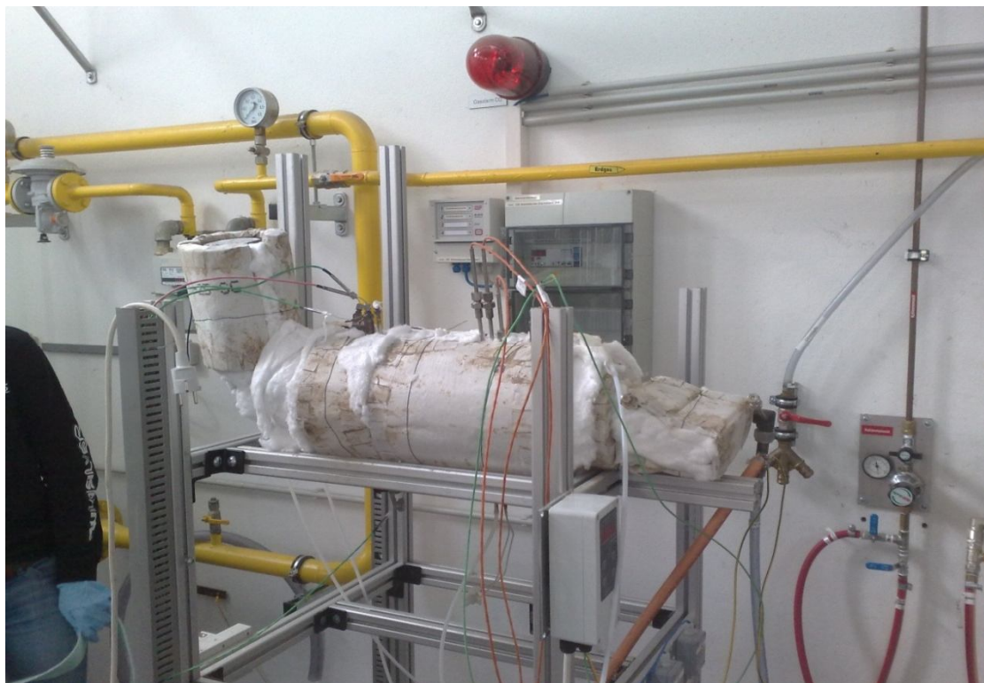
Fig.4.9 The T-POX reformer (first version) insulated with the main insulation layers.
