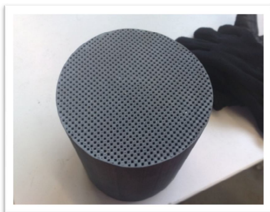
Fig.4.5 The soot trap by SiSiC ceramic material.
