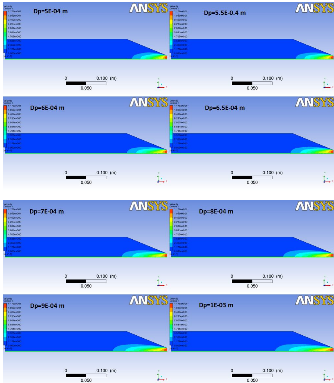
Fig. 3.18: Air stream propagation in the porous medium domain for different values of porous medium particle diameter, inlet velocity 11,7 [m/s] and temperature 293.15 [K].
