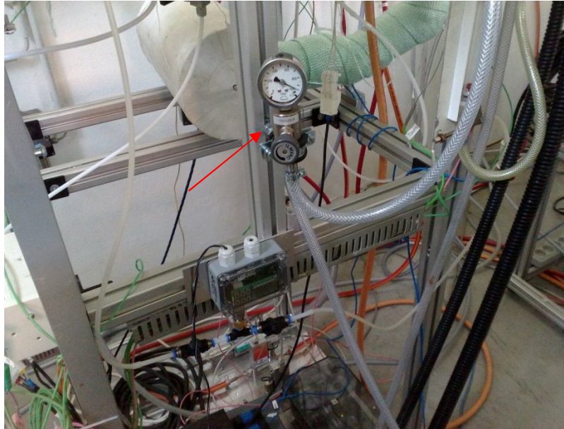
Fig. 4.36: The pressure reducer valve
