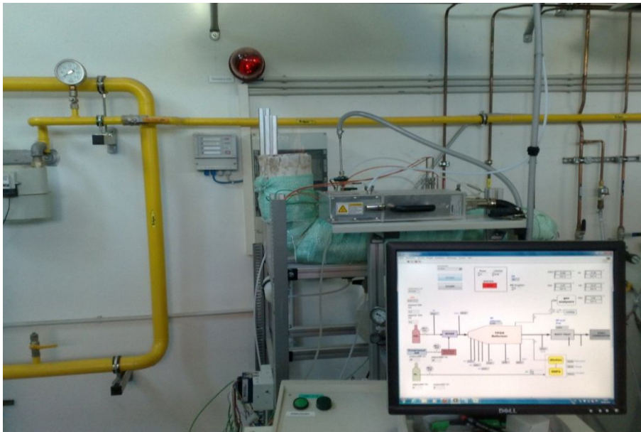
Fig.4.18 The Lab-View software for the controlling and observation of the experiment conditions
