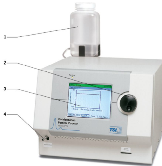
Fig. 4.26: Condensation Particle Counter with 1 Storing tank for butanol; 2 Control panel; 3 Display; 4 Input monodisperse aerosol.
