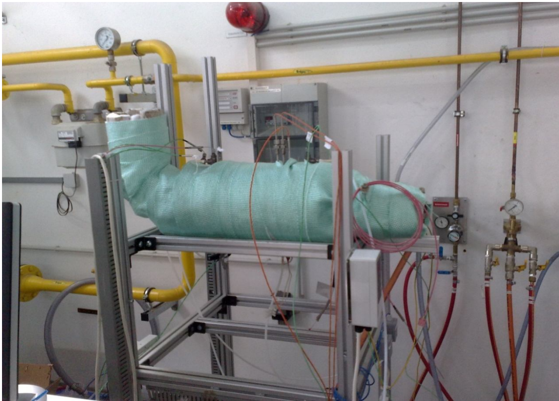
Fig.4.10 The T-POX reformer (first version) with the final insulation.
