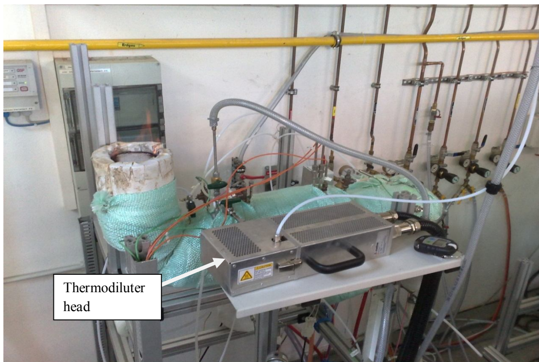
Fig.4.11 The final assembly (second version) with the thermodiluter head of dilution system which is analyzed thoroughly in the paragraph 4.1.5.
