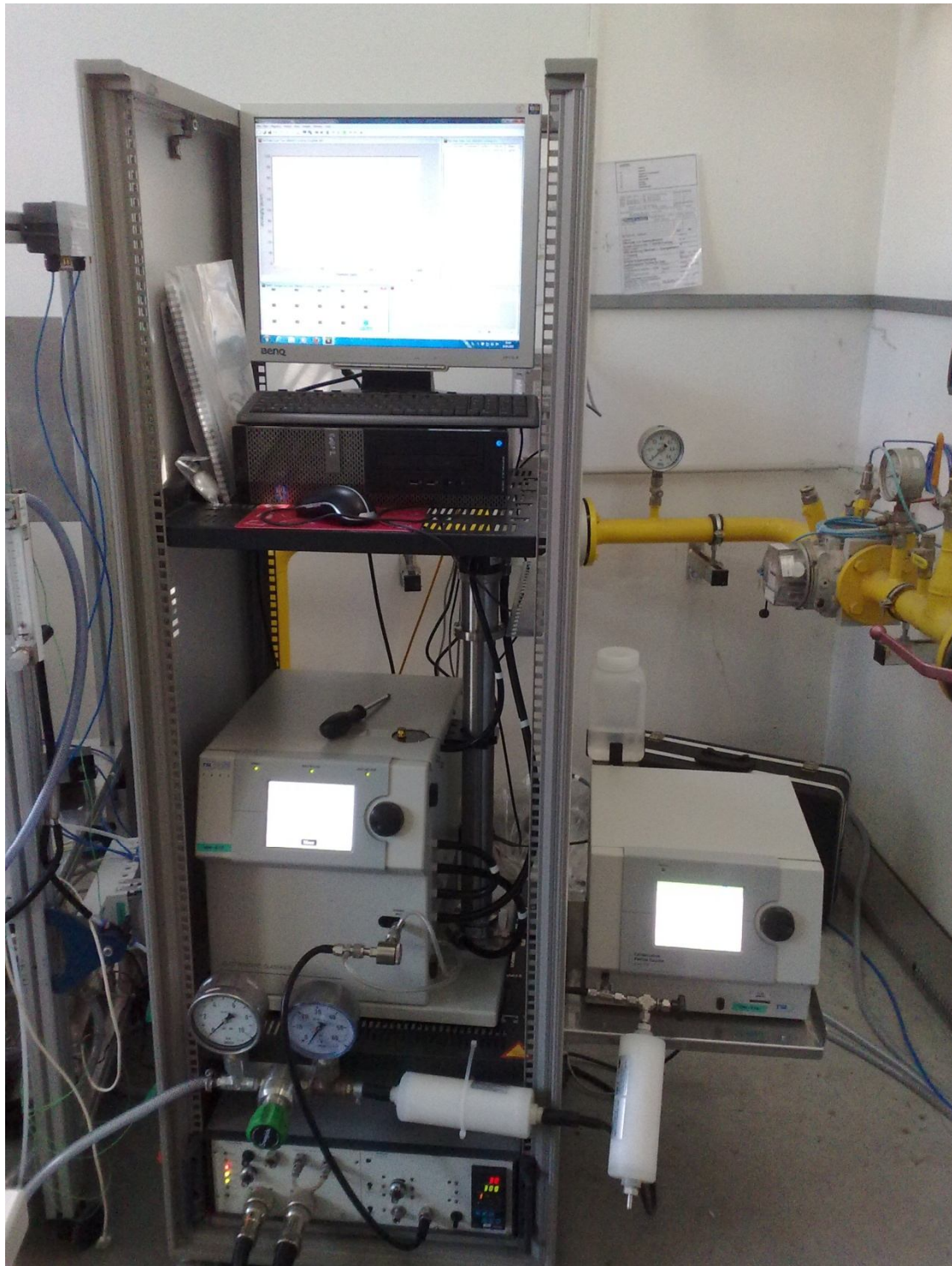
Fig.4.27 The SMPS system which were conducted the soot measurements in this study, in the laboratory of Technical University Bergakademie of Freiberg in Germany.
