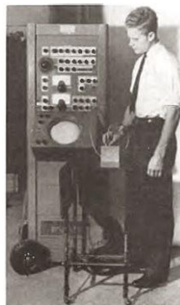
FIG. 2a. Type A supersonic reflectoscope.
