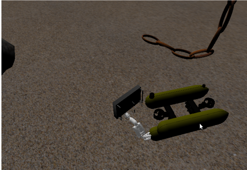
Figure 4.13: 1 st Solution Process - Case Study 2: UVMS final optimal pose configuration grasping the valve head.
