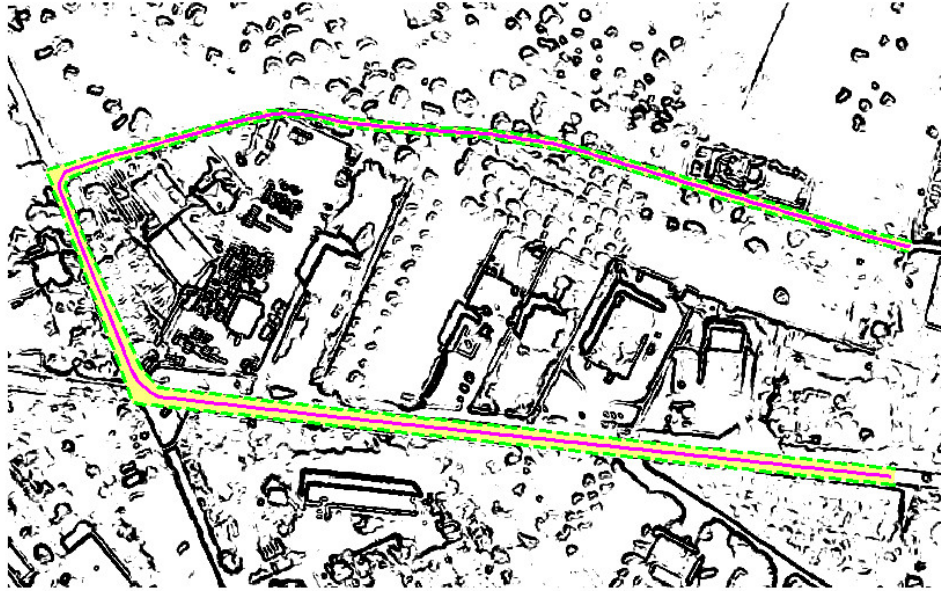
Figure 5.4: Image with Sobel filter: road edges (green), road centreline (magenta).
