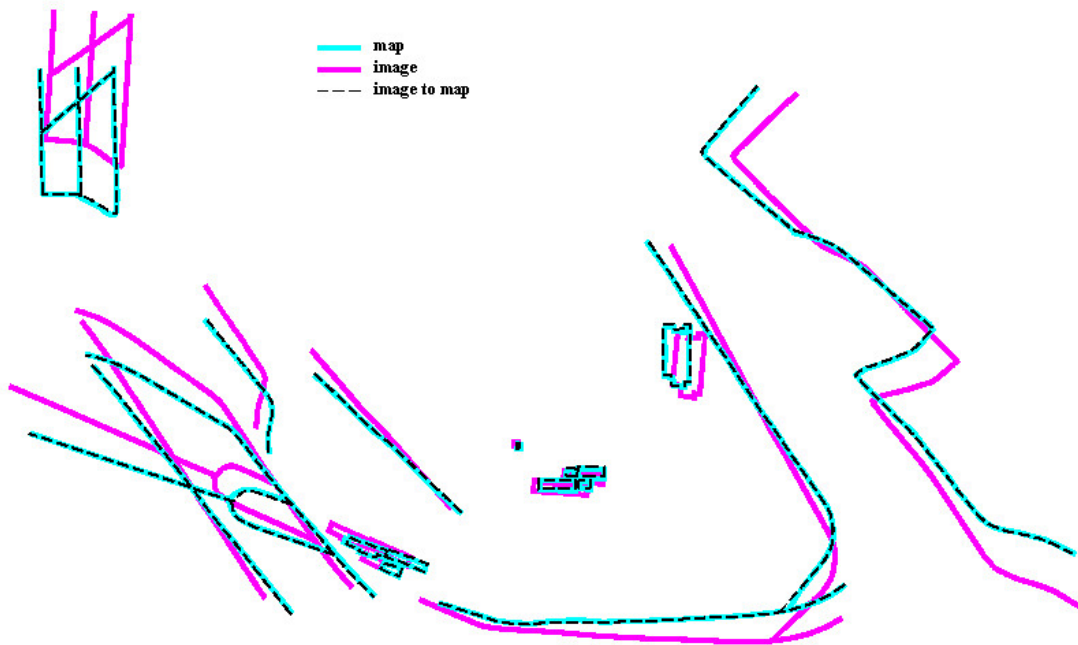
Figure 5.33: Registration using linear features: pre-aligned data and results.
