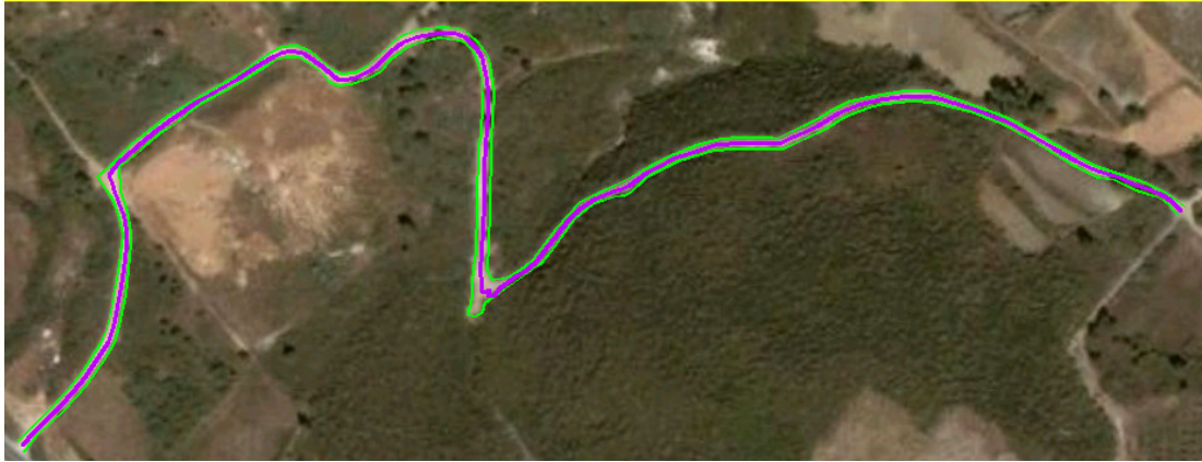
Figure 6.22: Optical: road edges (lines in green), road centreline (in magenta).
