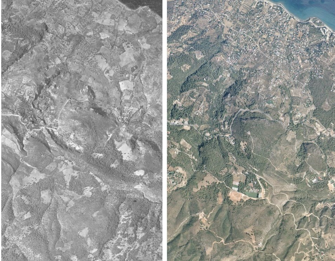
Figure 5.39: Data sets: aerial photograph captured in 1945 (left), orthoimage made from aerial images collected in 2008 (right).
