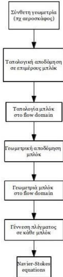
Fig.7: General structure for solving a CFD problem.
