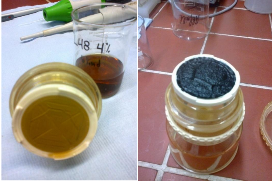
Pic. 7: Membrane after filtration without activ. carbon (left) and with activ. carbon (right).
