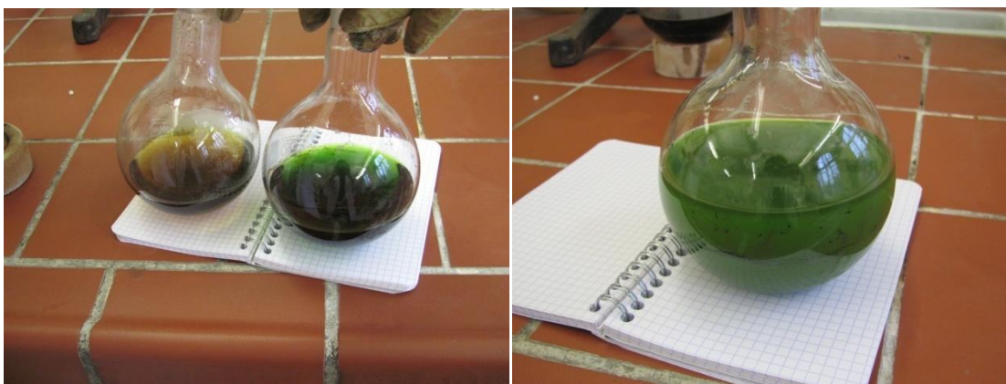
Pic. 11: Soxhlet extracts with water and EtOH (left), EtOH after adding 200mL water (right).
