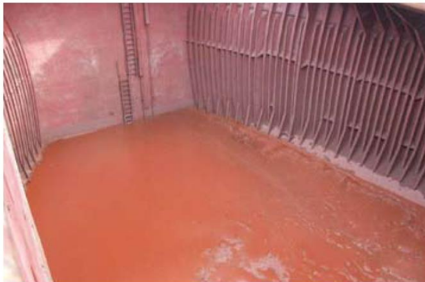
Figure 1.2: Cargo hold with wet iron ore fines
