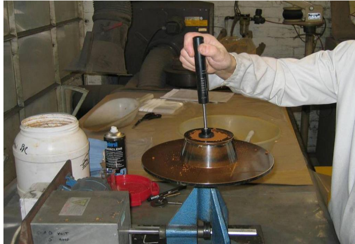
Figure 3.3.1: Flow Table Testing of nickel ore. Filling the mould and tamping procedure Preparation of the test samples
