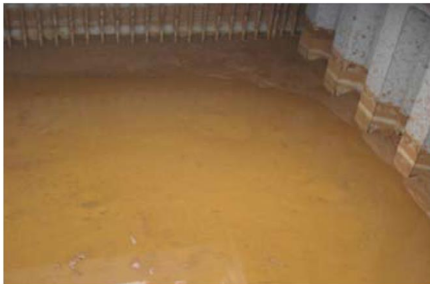
Figure 1.3: Cargo hold with wet nickel ore cargo
