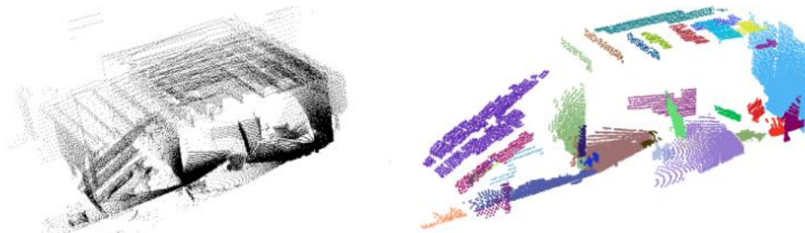
(e) Failed alignment of scans 6-7 – Visualization using points (f) Failed alignment of scans 6-7 – Visualization using planar segments
