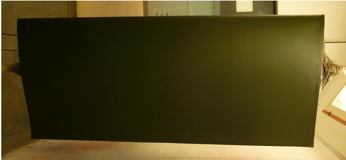
Figure 5: The wing model after being painted with a mat black dye with Rhodamine 6G. View of the pressure side.
