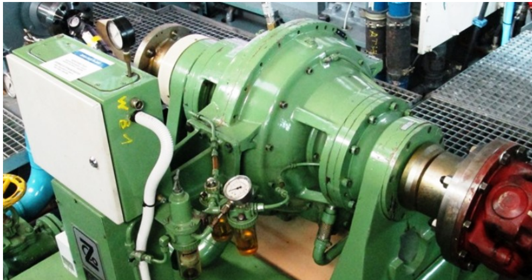
Figure 3.22: Water Brake at LME - view from coupled end
