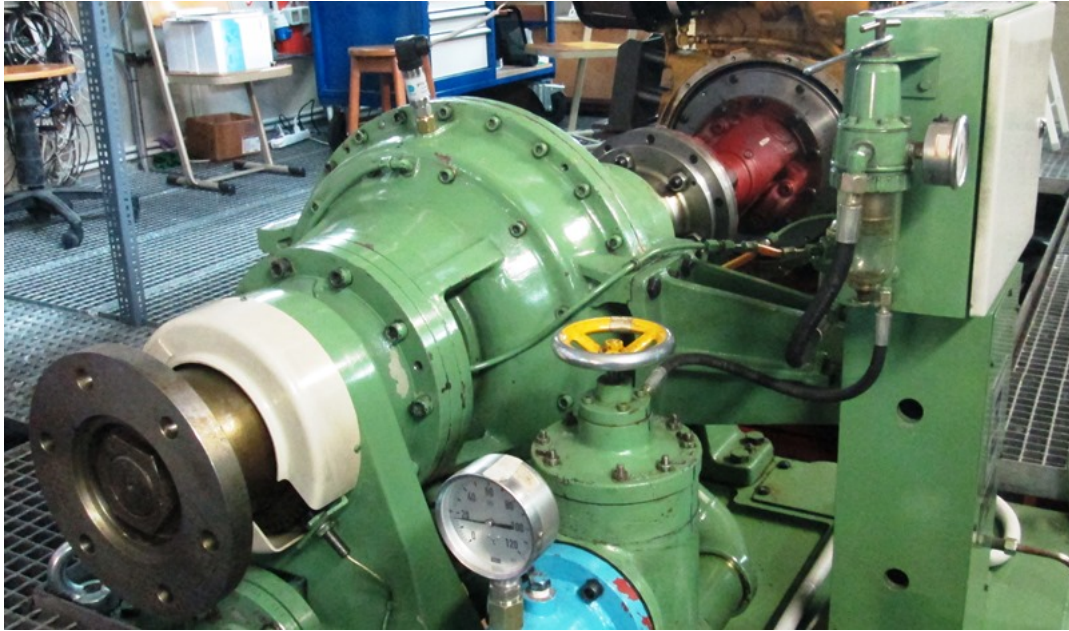
Figure 3.19: Water Brake at LME - view from free end
