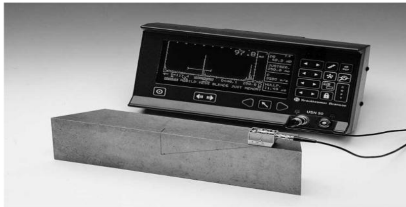
Fig. 55 USN 50: A hole being scanned with the probe MWB 60-4E
