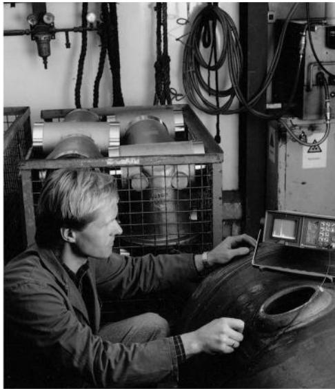
Fig. 14 Ultrasonic Testing in practice.
