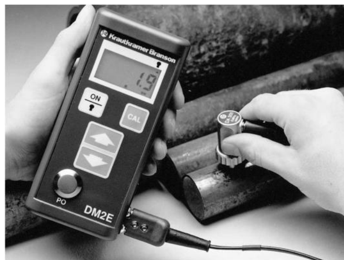
Fig. 38 Wall thickness measurement with a digital thickness gauge in practice.
