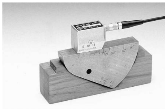
Fig. 47b MWB 45-4E on Calibration Block 2
