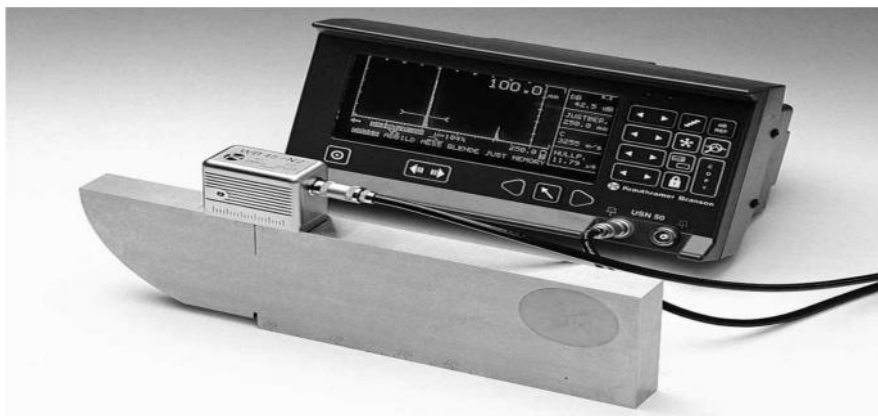
Fig. 50 Range: 250 mm with a WB 60-2 on V1 block
