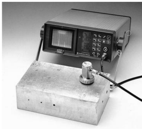
Fig. 43 USK 7 D: Calibration of a 250 mm range with an 80 mm aluminum path.
