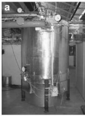
Equipment for thermal and catalytic treatment of waste gases polluted by carbon monoxide, VOC and \text{NO}_x
