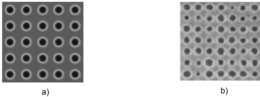
Figure 1.4 a) Printed contact holes with low dimensional variability and high Local Critical Dimension Uniformity and b) Printed contact holes with high variability (low LCDU)
