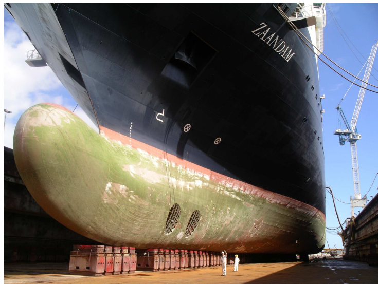
Figure I.7: A bulbous bow with a complex shape. Source: commons.wikimedia.org.
