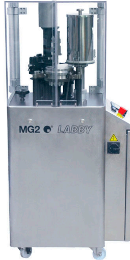
Figure 2.4: MG2 capsule filling lab scale (LABBY)
