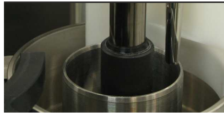
Figure 4.2: The rotary container-MG2 LABBY
