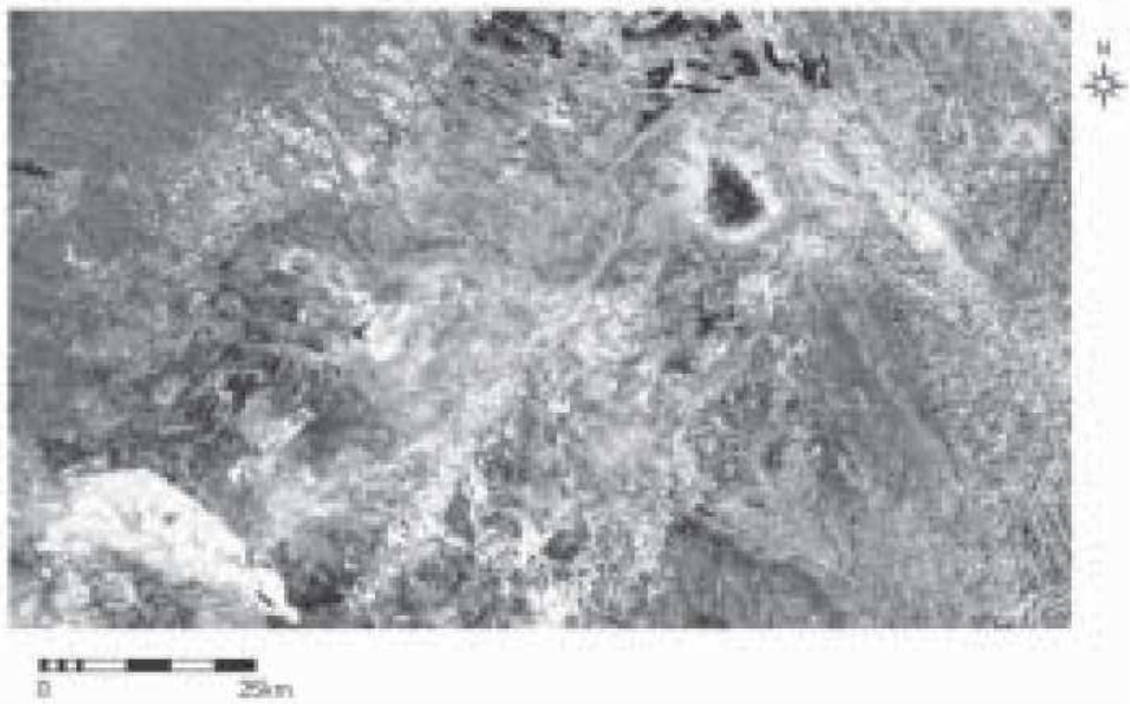
Figure 4: Fourth principal component showing hydroxyl as bright pixels
