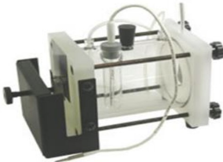
Fig 48. The three-electrode cell of our lab, Model K0235 Flat Cell
