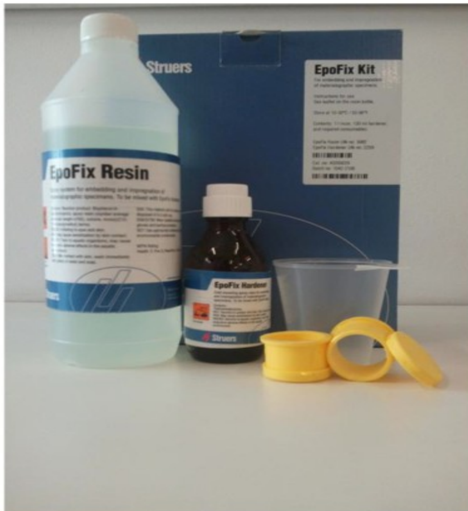
Fig. 39. Epofix Kit: Resin, Hardener, Mounting cup, Mixing cup
