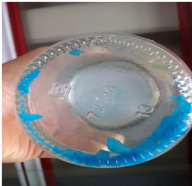
Fig. 52. Image of the super-hydrophobic film remains at the bottom of the solution
