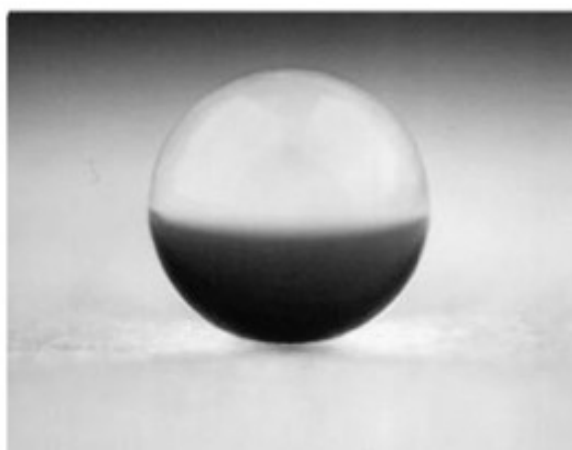
Fig. 4. A water droplet of which the contact angle is 174^\circ placed on the AKD surface [3]
