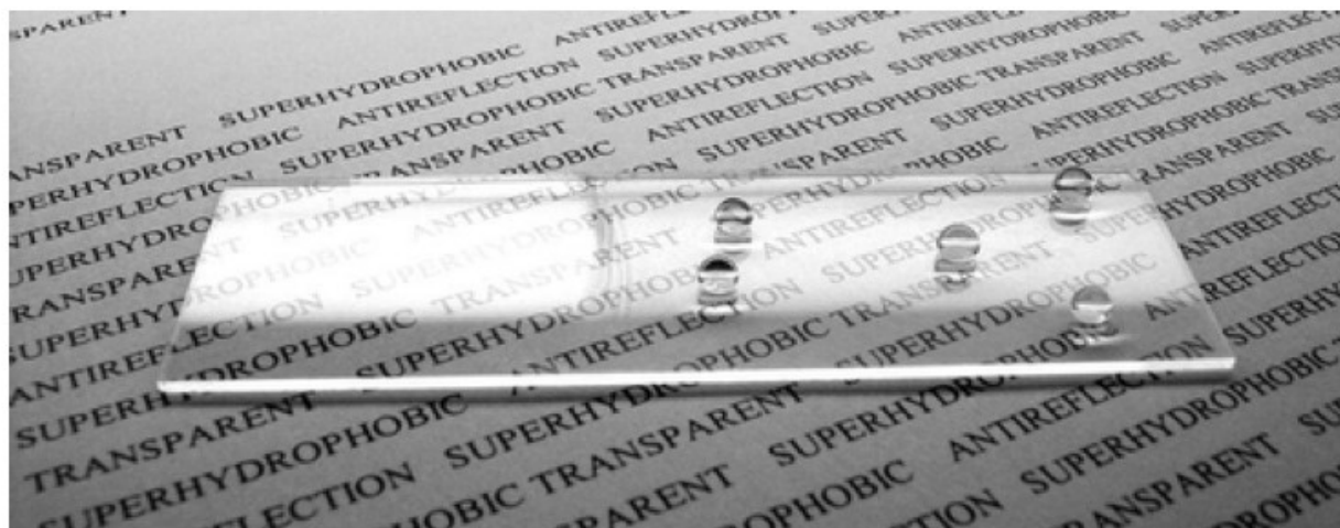
Fig. 36. Image of a glass slide coated with a transparent, superhydrophobic multilayer with antireflection properties [16]
