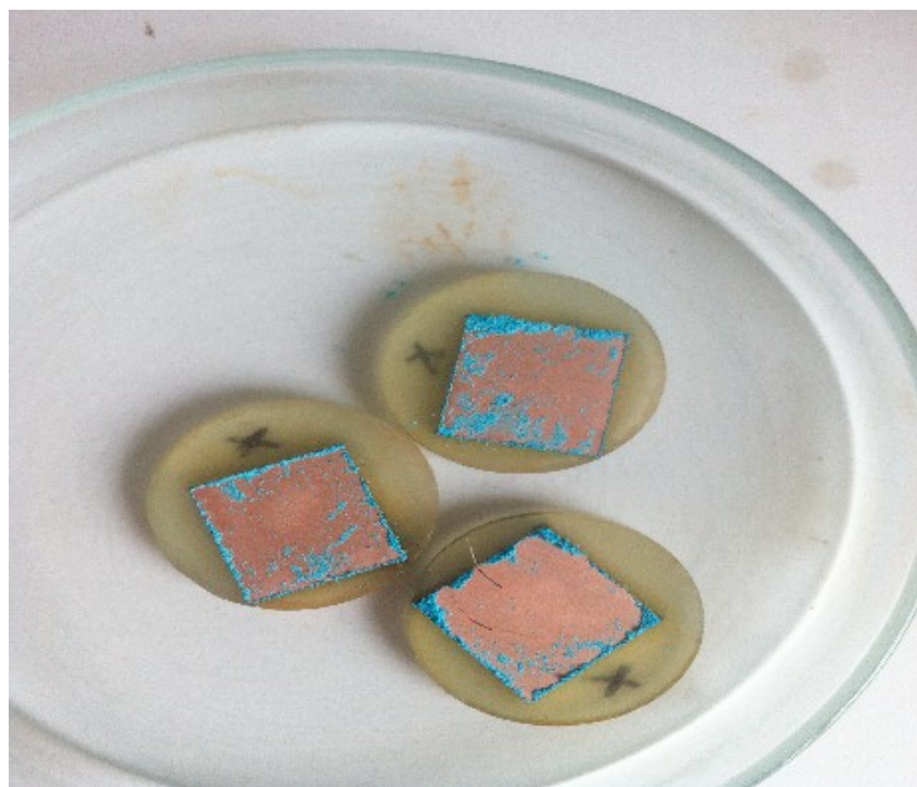
Fig. 51. Image of specimens treated in 0.09M myristic acid, unsuccessful CSD method, abruption of the Super-hydrophobic film
