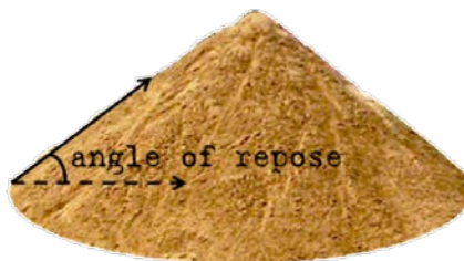
Figure 3.7 Definition of repose angle of a granular material
