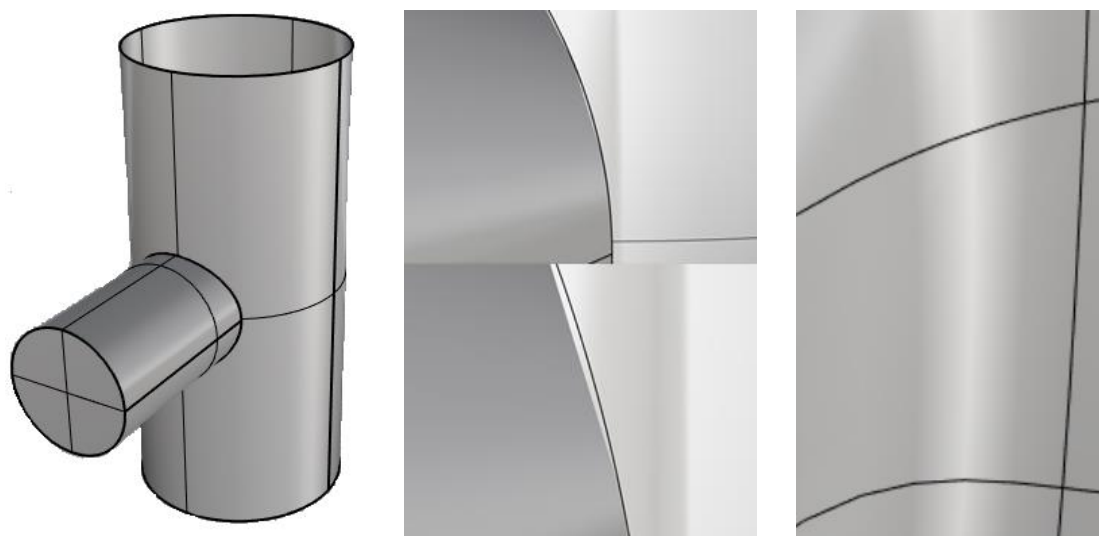
Figure 5.7. T-Spline model. Watertight patch interconnection.
