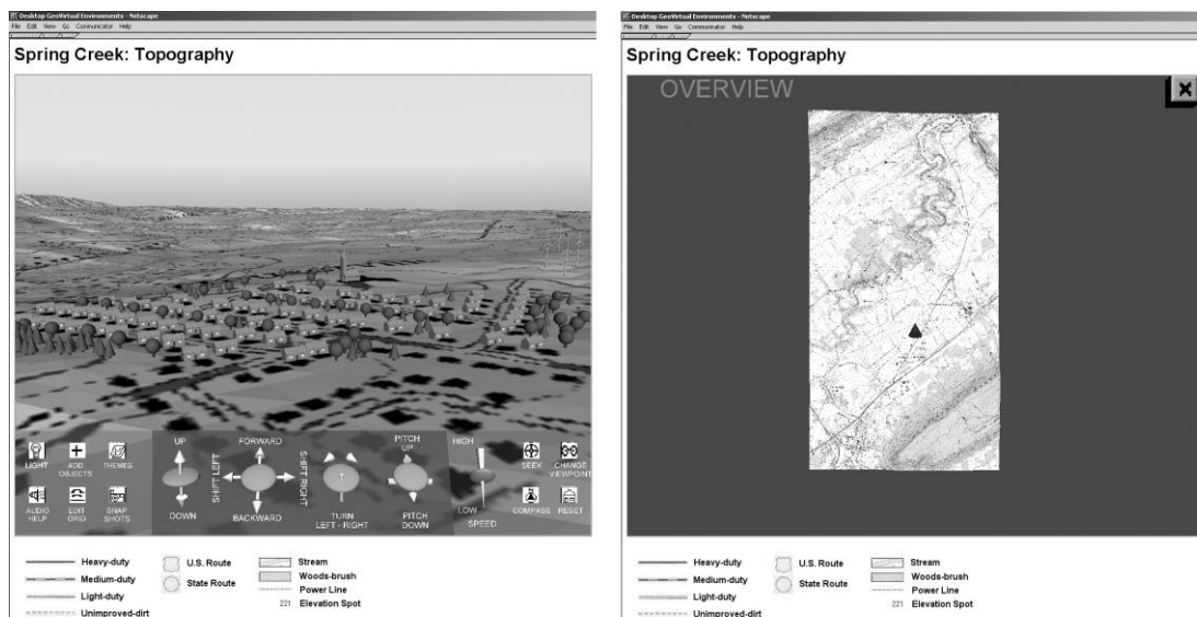
Figure 32: Example of combining 3-d egocentric with linked 2-d exocentric perspectives leading to the enhancement of user navigation and orientation. After Fuhrmann, 2003.
