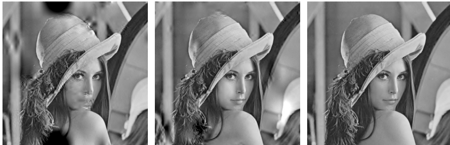
(α) \alpha = 1 , PSNR = 18.2\text{dB} , C/N_0 = 13.6\text{dB} (β) \alpha = 4 , PSNR = 22.58\text{dB} , C/N_0 = 13.6\text{dB} (γ) \alpha = 1 , PSNR = 35.19\text{dB} , C/N_0 = 25.6\text{dB}
