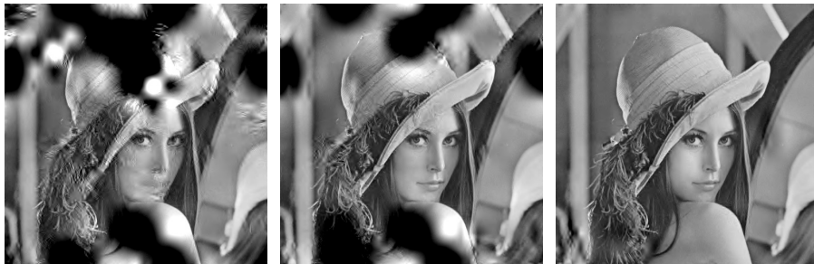
(α) \alpha = 1 , PSNR = 7.76\text{dB} , C/N_0 = 19.8\text{dB} (β) \alpha = 1.75 , PSNR = 9.67\text{dB} , C/N_0 = 19.8\text{dB} (γ) \alpha = 1 , PSNR = 34.54\text{dB} , C/N_0 = 32.1\text{dB}
