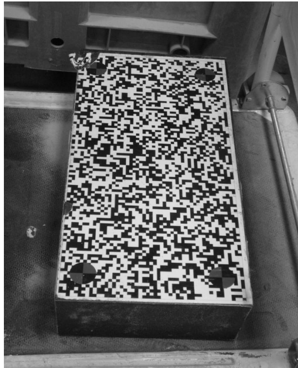
Figure 3.3. Photographs of the caisson model. The side tangent to the glass is covered with a pattern for image analysis purposes.
