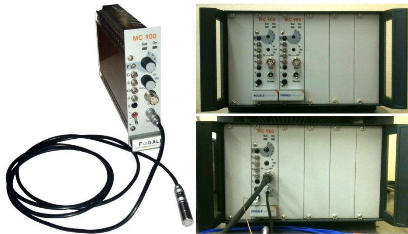
Figure 2. 9: Fogale MCC-10 attached to MC900 (left) and the modules at hand (right)
