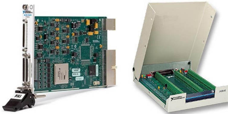
Figure 2. 18: PXI-7841R (left) and SCB-68 connector block (right)
