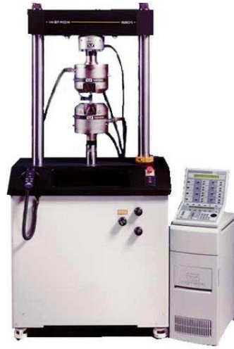
Figure 2. 4: Instron 8516 servo-hydraulic fatigue system
