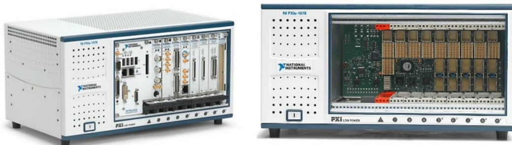
Figure 2. 13: Images of a populated and an unpopulated PXIe-1078 chassis
