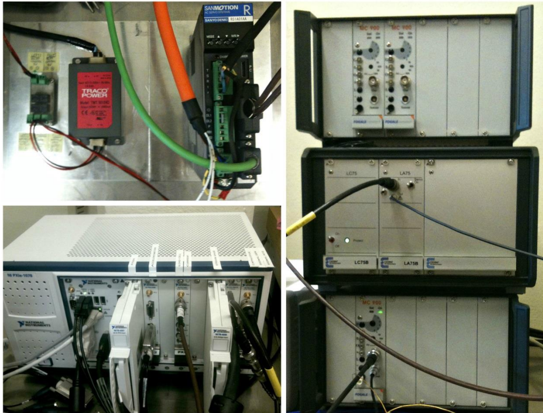
Figure 2. 2: Peripheral devices- National Instruments PXI chassis and modules (bottom-left), motor servo amplifier and mechanical brake power supply (top-left) and stack of linear amplifier for piezo actuators and capacitive measurement modules (right)
