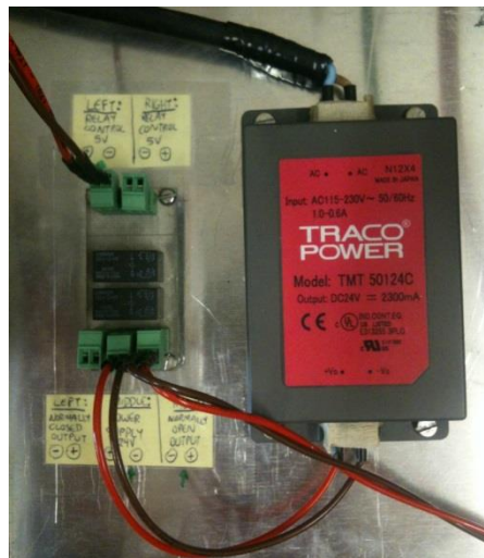
Figure 2. 19: Relay board and external power supply used to control the motor brake
