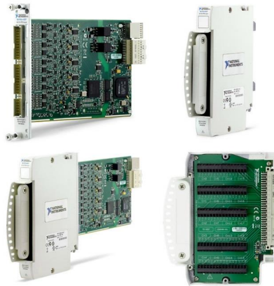
Figure 2. 15: PXIe-4357 (top-left), TB-4357 (top-right), TB-4357 connected to PXIe-4357 (bottom-left) and TB-4357 innards (bottom-right)
