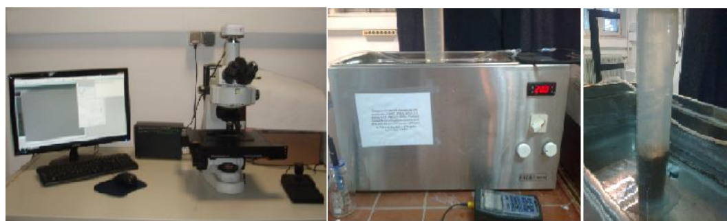
Figure 1: Left: Optical Microscope Nikon Eclipse 80 and Video camera Lumenera Infinity 1-3c (2048x1536 pixel, 24 bit) used for capturing of activated sludge images by using the software Image Pro Plus, Right: Experimental Procedure in order to estimate the parameters that are related to sludge settleability and compactability like the Diluted Sludge Volume Index (DSVI), the zonal settling velocity and the Vesilind's parameters V_0 and n .
