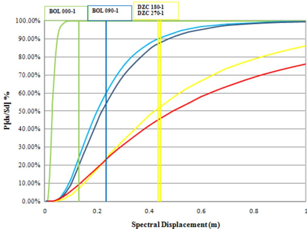
Figure 8.17 Fragility curves showing damage limit state for recording station in Duzce, Turkey
