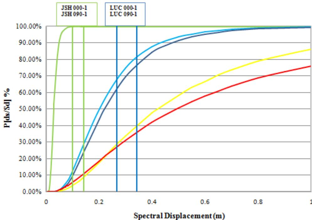
Figure 8.4 Fragility curves showing damage limit state for recording station in Landers, USA
