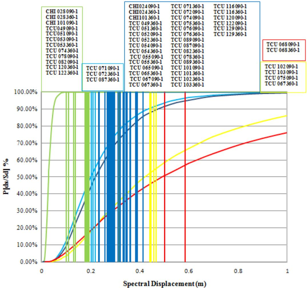
Figure 8.15 Fragility curves showing damage limit state for recording station in Chi-Chi, Taiwan
