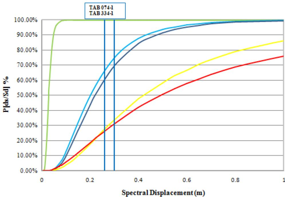
Figure 8.11 Fragility curves showing damage limit state for recording station in Tabas, Iran
