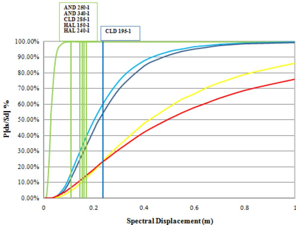
Figure 8.7 Fragility curves showing damage limit state for recording station in Morgan Hill
