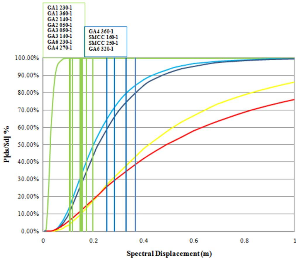
Figure 8.16 Fragility curves showing damage limit state for recording station in Coyote Lake, USA
