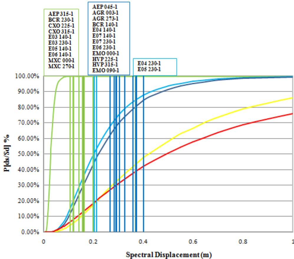
Figure 8.2 Fragility curves showing damage limit state for recording station in Imperial Valley, USA, 1979
