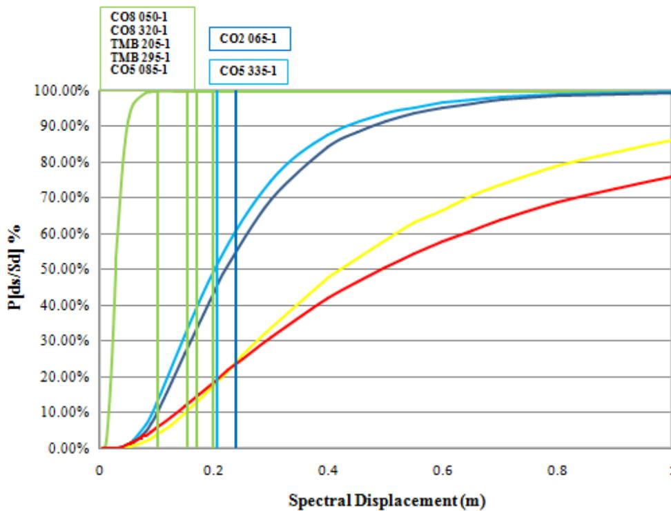
Figure 8.14 Fragility curves showing damage limit state for recording station in Parkfield, USA
