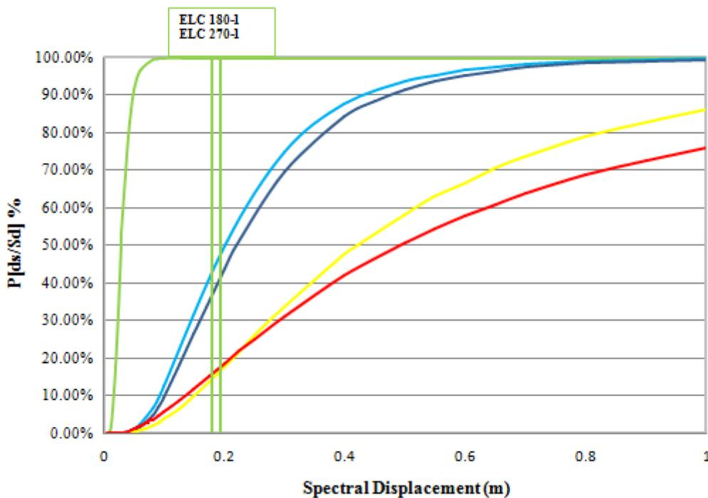
Figure 8.1 Fragility curves showing damage limit state for recording station in Imperial Valley,USA, 1940
