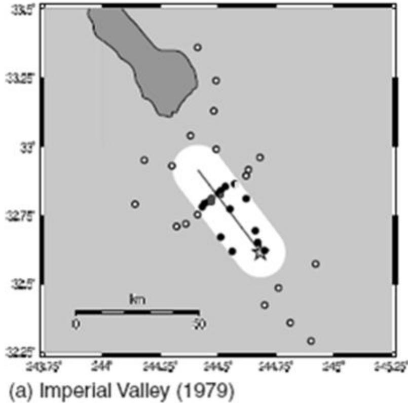
Figure 8.1 Map of stations in relation to the rupture of the earthquake area in IMPERIAL Valley, CA, USA, 1979
