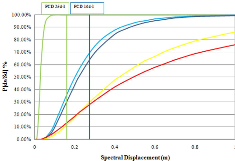
Figure 8.12 Fragility curves showing damage limit state for recording station in San Francisco
