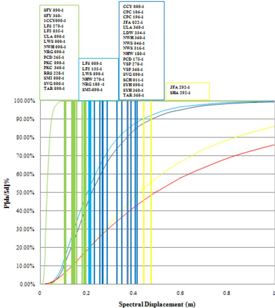
Figure 8.21 Fragility curves showing damage limit state for recording station in Northridge, USA
