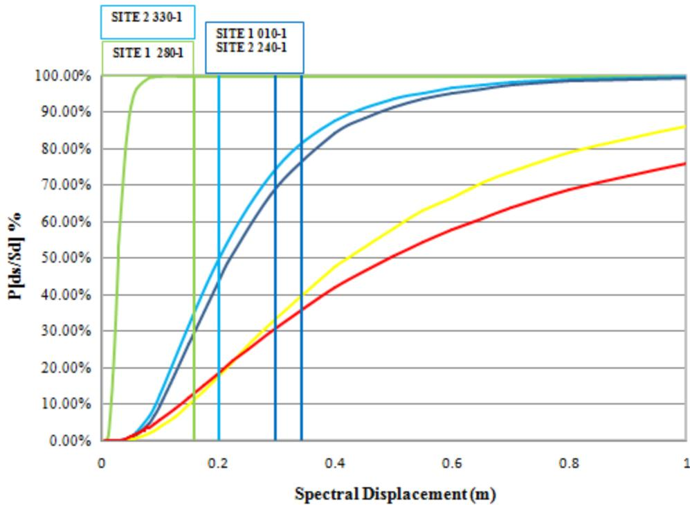
Figure 8.8 Fragility curves showing damage limit state for recording station in Nahani River, Canada
