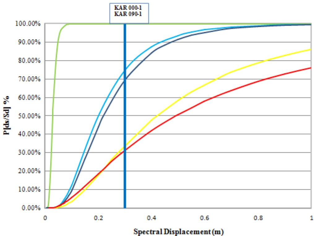
Figure 8.19 Fragility curves showing damage limit state for recording station in Gazli, URSS
