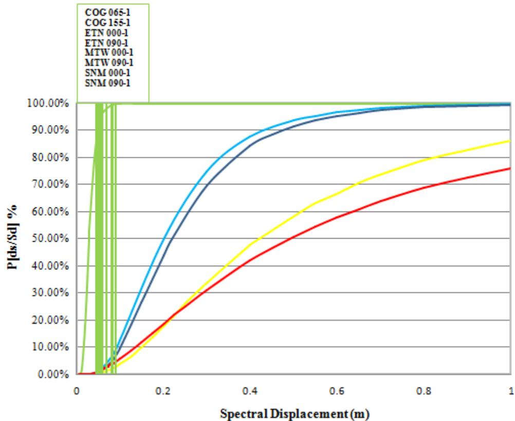
Figure 8.13 Fragility curves showing damage limit state for recording station in Sierra Madre
