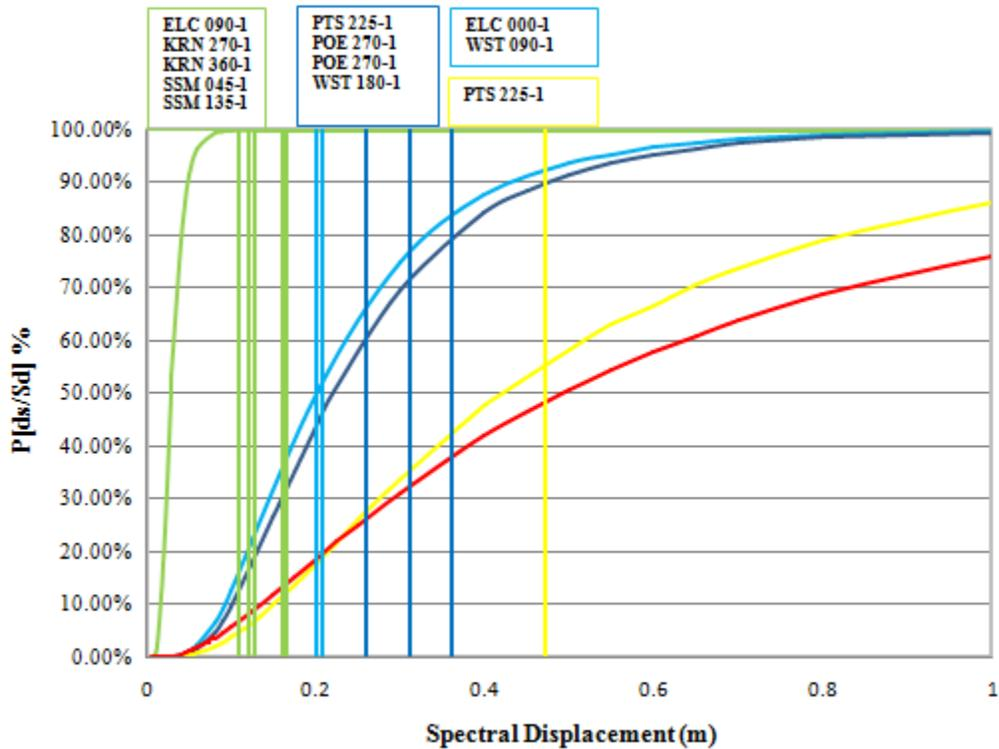
Figure 8.10 Fragility curves showing damage limit state for recording station in Superstition Hills
