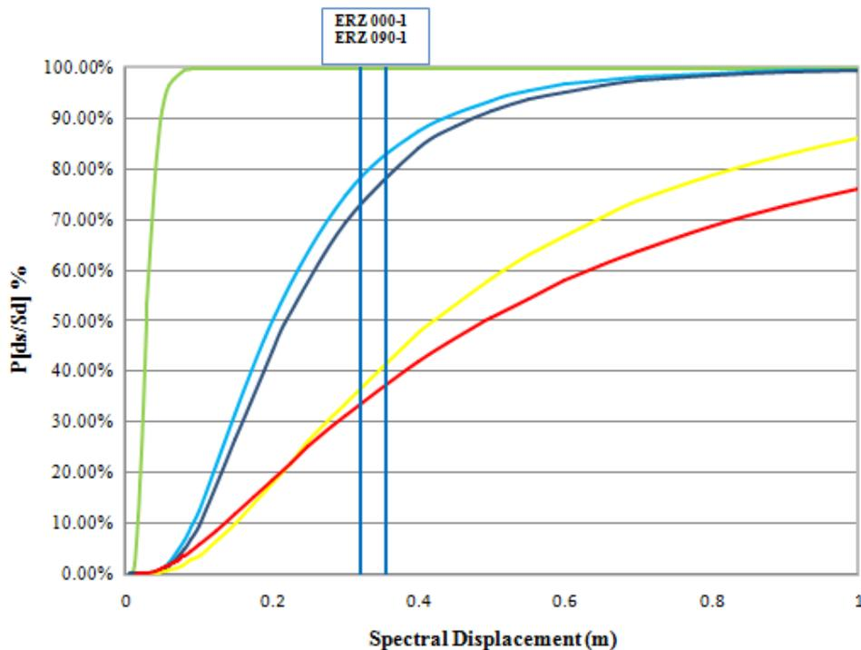
Figure 8.18 Fragility curves showing damage limit state for recording station in Erzican, Turkey
