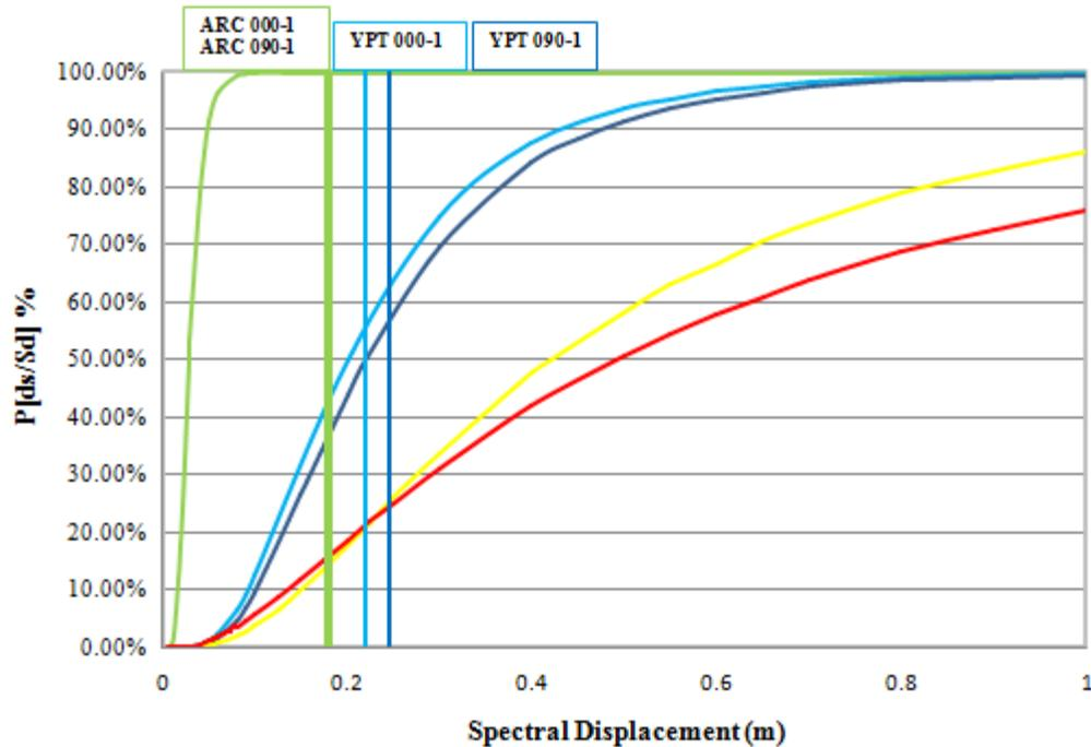
Figure 8.3 Fragility curves showing damage limit state for recording station in Izmit, Turkey
