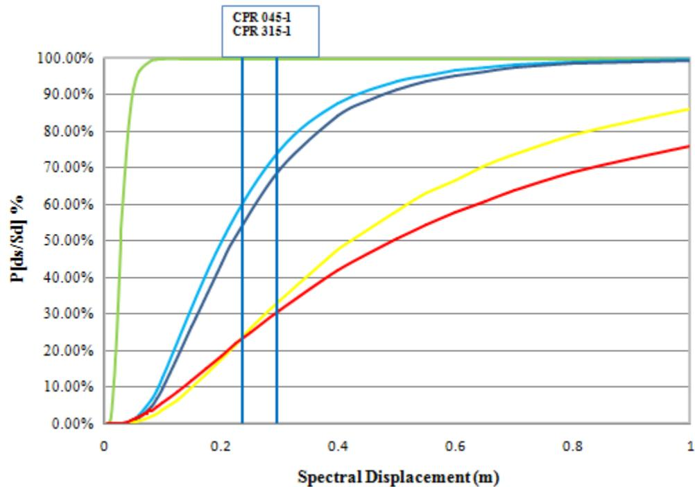
Figure 8.6 Fragility curves showing damage limit state for recording station in Mexicali Valley
