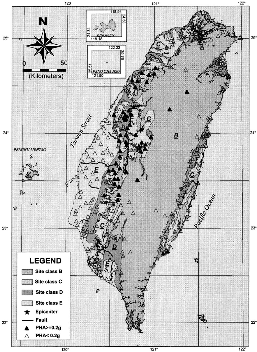
Map 8.6 map showing the 441 acceleration recording stations. Because some stations have more than one recorder accelerograph, essentially there are 412 stations. Among the 441 stations, 56 of them which are indicated by a solid black triangle, show the stations to record maximum horizontal ground acceleration greater than 0.2 g.
