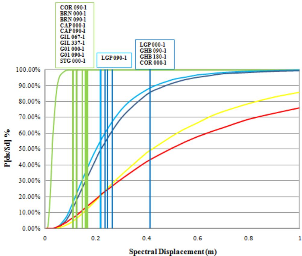
Figure 8.5 Fragility curves showing damage limit state for recording station in Loma Prieta
