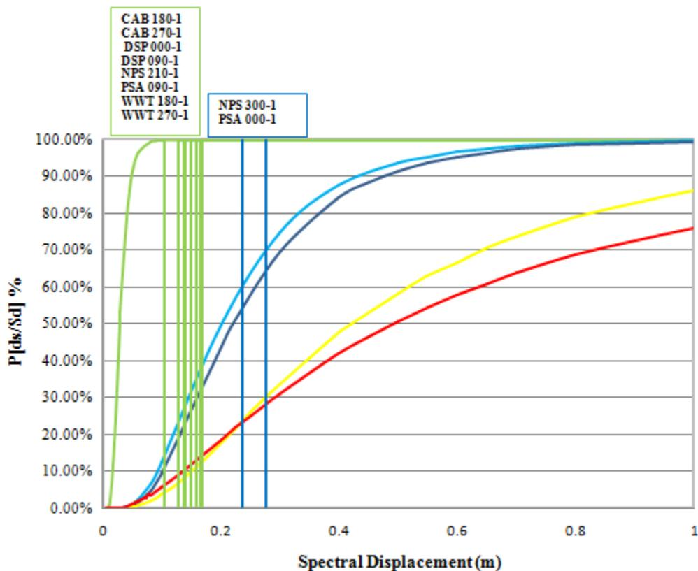
Figure 8.9 Fragility curves showing damage limit state for recording station in Palm Springs
