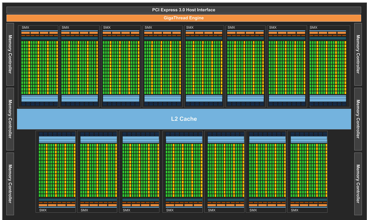
Fig. 4.4: NVIDIA Kepler (GK110) GPU block diagram
