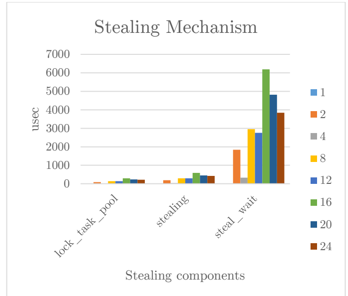
Figure 126. Matrix multiplication scalability of stealing components on NUMA for each thread count
