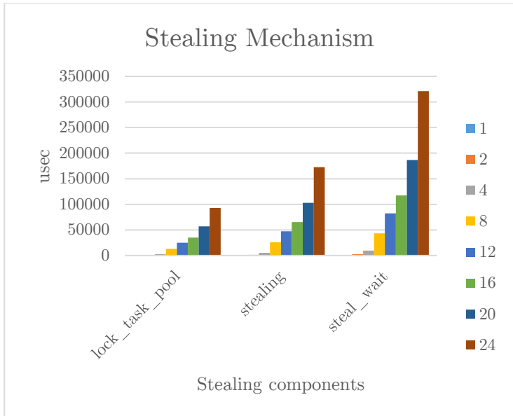
Figure 137. Convex Hull scalability of stealing components on SMP for each thread count
