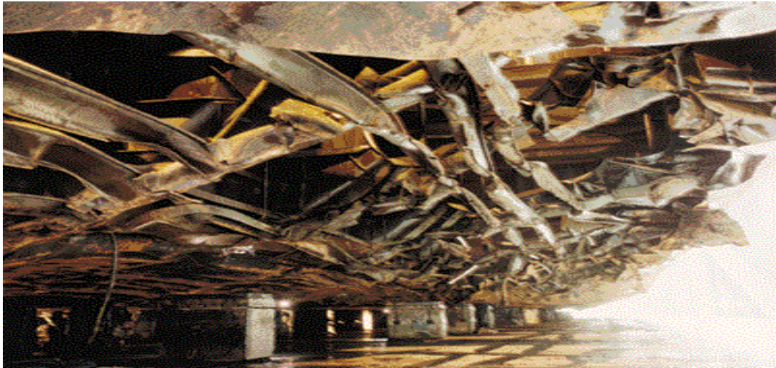
Σχήμα 35 The bottom of the M/V Sea Empress after the grounding (Samuelides et al, 2007)
