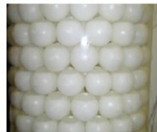
(vi) Fixed bed arrangement with PCM balls
