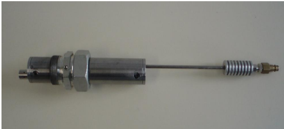
Figure 4.6.3. Heat extractor fitted to the trial air - curtain
