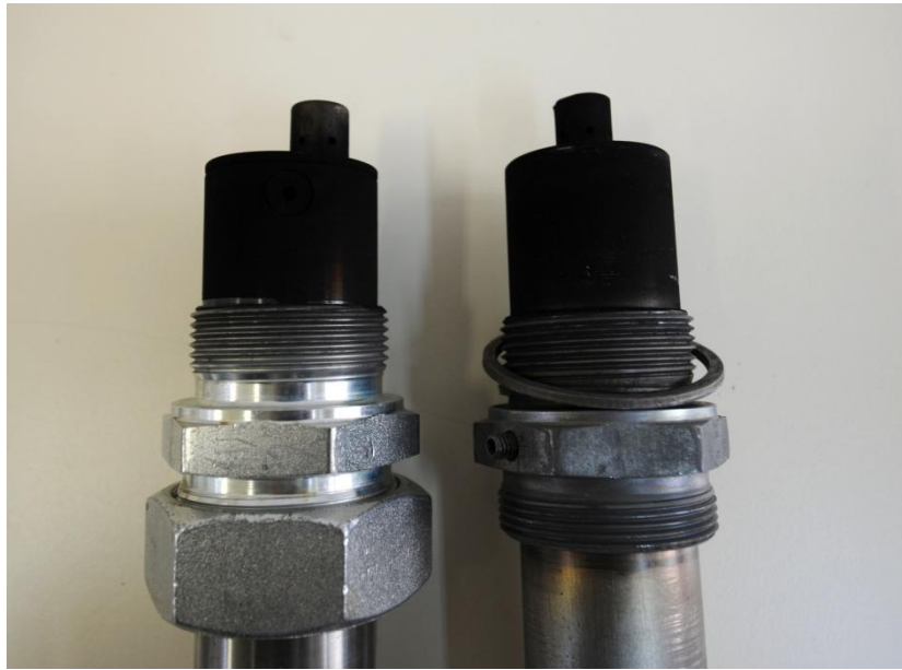
Figure 7.5.4. SNS (left) and dummy SNS (right) after two hours of engine operation.
