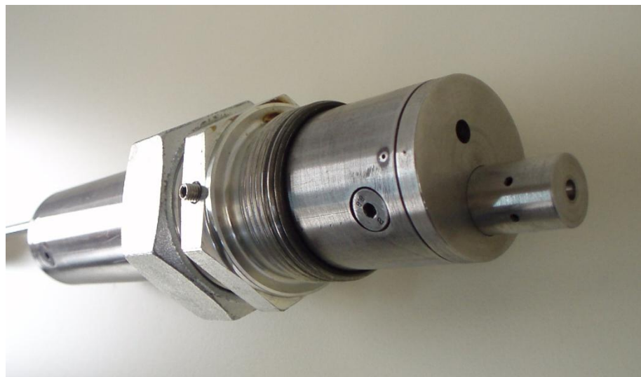
Figure 3.2.8. Trial air curtain device with axial nozzle
