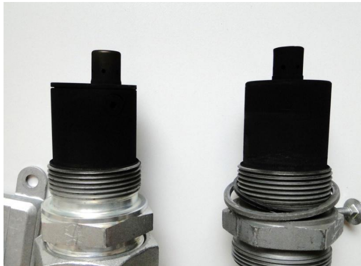
Figure 7.5.13. SNS (left) and dummy SNS (right) after eight hours of engine operation.
