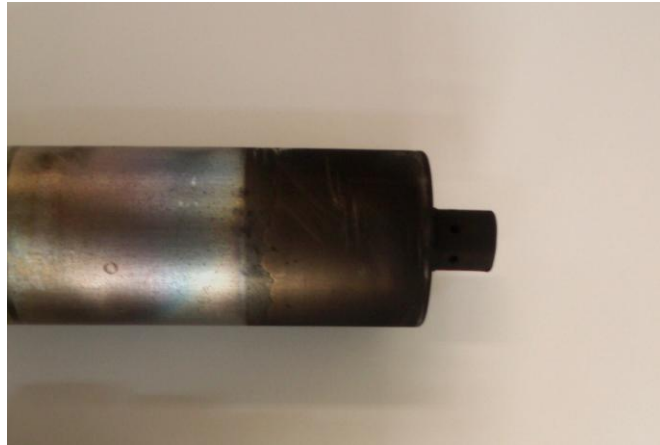
Figure 4.6.2. Dummy SNS after two hours of engine operation.
