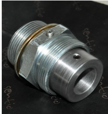
Figure 4.3.4. Adaptor for installation of velocity meter.
