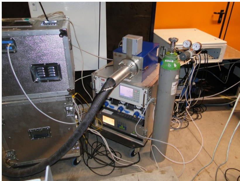
Figure 7.2.2. A. CLD analyzer's front panel during calibration procedure. B. CLD analyzer during span gas supply
