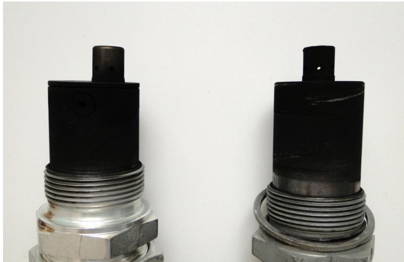
Figure 7.5.10. SNS (left) and dummy SNS (right) after six hours of engine operation.
