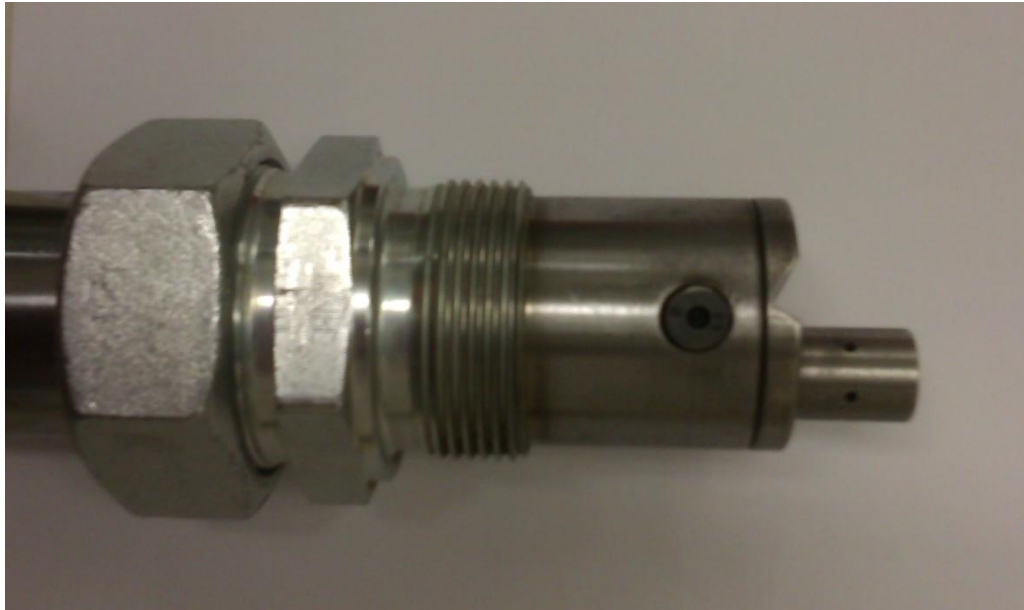
Figure 3.3.3. Trial air curtain device with inclined nozzle
