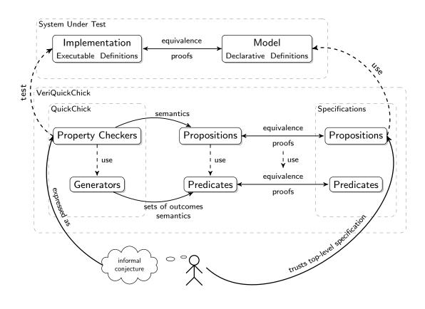
Figure 1.1: The proposed verification methodology
