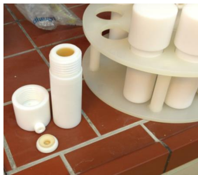
Figure 14: The digestion vessels with the pressure protection caps.
