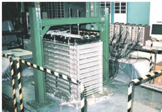
Figure 3.38: Apparatus used in the experimental investigation of the effectiveness of the screen pipe method.
