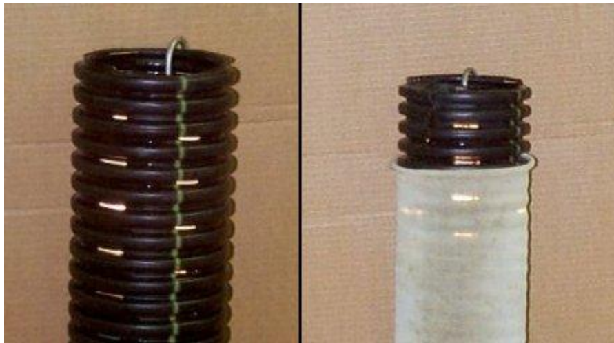
Figure 3.1: Corrugated pipe without filter fabric (a) and enclosed in filter fabric (b) (Nilex Inc.; personal communication).
