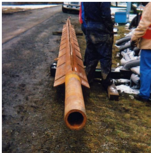
Figure 3.3: Tubular steel mandrel for EQ-drain installation (left figure) and dimension specifications (Nilex Inc.;personal communication).
