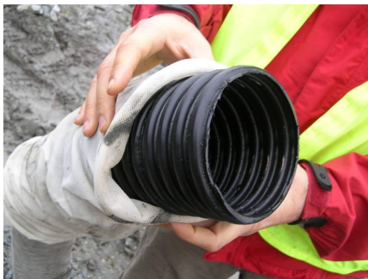
Figure 3.2: EQ-drain ready to be installed (after E. Naesgaard; personal communication).
