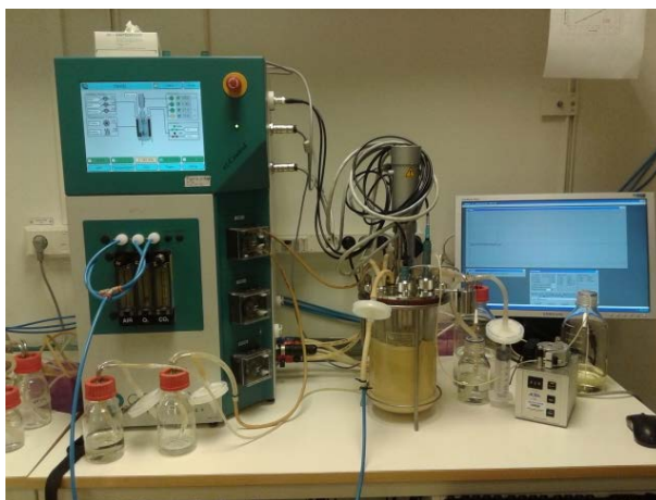
Figure 7.3. Fermentation of Pichia pastoris recombinant strains was carried out in a 3 lt glass autoclavable Applikon bioreactor, equipped with an ez -Control system (Applikon Biotechnology B.V., Netherlands). Glycerol and methanol feeding was performed with Alitea XV pump with MasterFlex 96400 L/S 14 silicon tube (glycerol) and PharmaMed 0.51mm (methanol).
