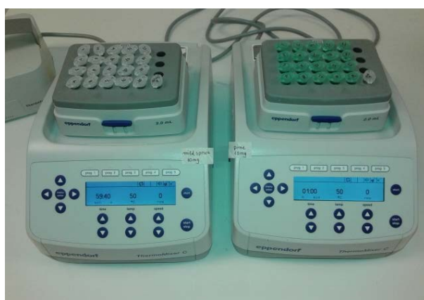
Figure 8.2. Enzymatic hydrolysis was performed in safe lock 2mL volume microtubes, with 1200 rpm agitation in Thermomixer incubator, which offers simultaneous mixing and temperature control (Eppendorf, Germany).
