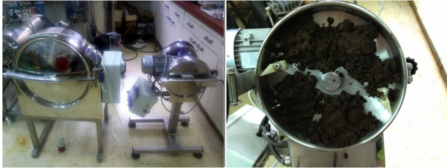
Figure 5.8 The laboratory scale liquefaction reactor based on fall mixing that was employed for the hydrolysis and the reduction of viscosity of PWS (18% w/w, DM) by the recombinant MtEG7a .
