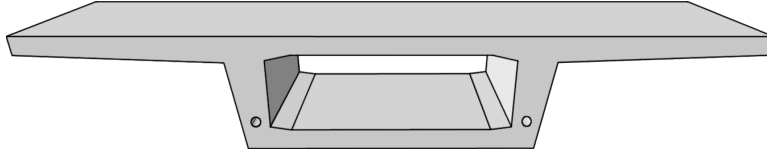
Figure 5.5: Prestressed concrete bridge part model
