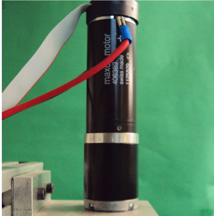
FIGURE 5.5: Maxon RE series motors fitted the MR type incremental encoders and planetary-gear transmissions.
