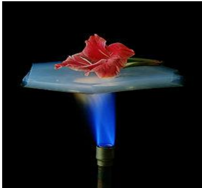
Fig 6. A flower on top of aerogel layer insulating the flame below [14]
