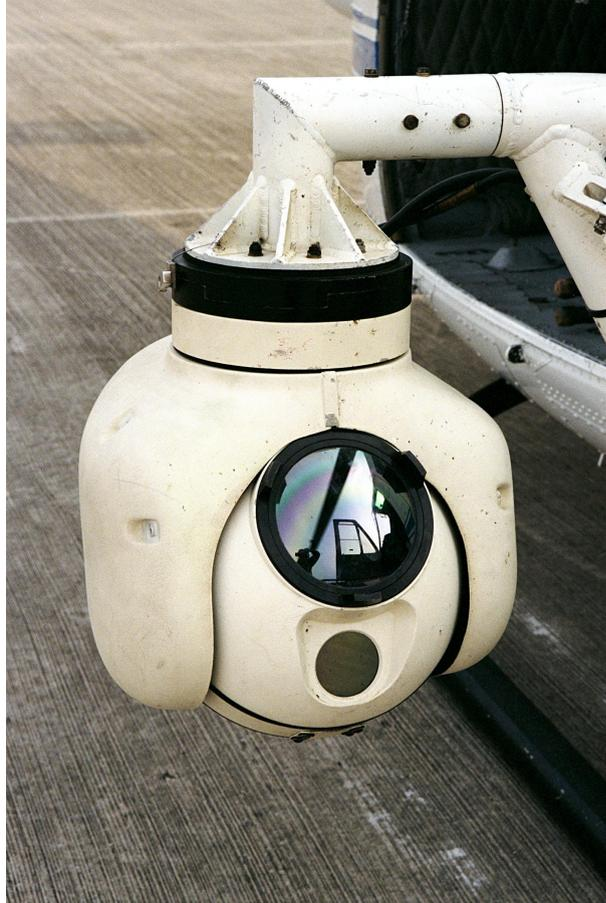
FIGURE 2.7: A thermal imaging gimbal pod camera mounted on the side of a Huey UH-1.
