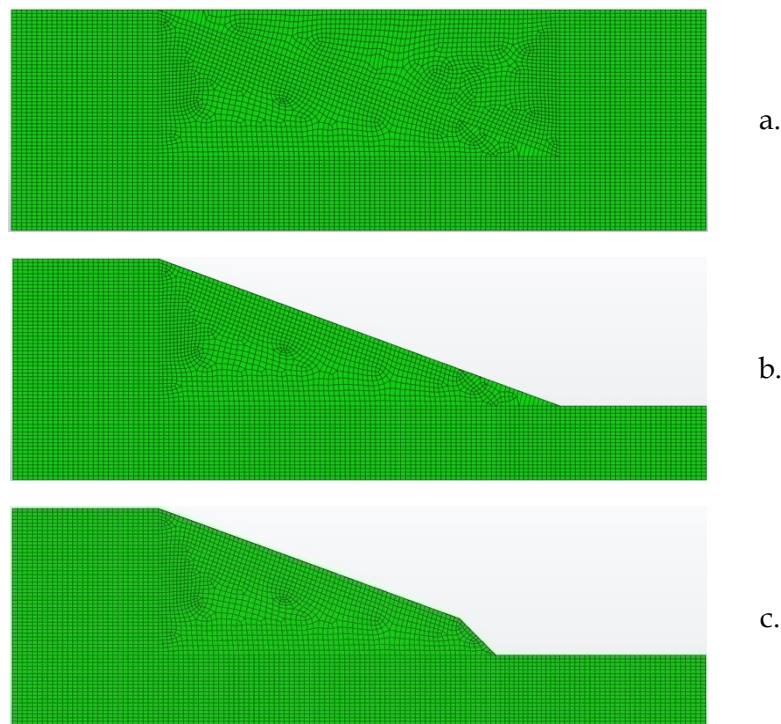
Figure 8.2: Schematic representation of the initial state and the following excavation steps: a. geostatic step; b. excavation of the initial slope and c. excavation of the final cut.
