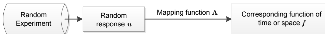
Figure 4.1: The sequence of events leading to assigning a stochastic function f to the response of a random experiment.
