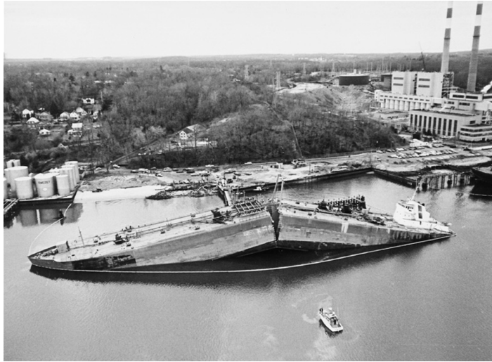
Figure 1.1: An oil tanker that fractured in a brittle manner by crack propagation around its girth (Callister and Rethwisch, 2012).
